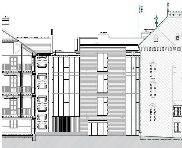
Extract from planning application drawing 2350-SJK-S2B-0-252 showing the north elevation of the proposed addition of a fully glazed 4-storey link building
