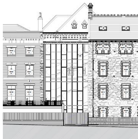
Extract from planning application drawing 2350-SJK-S2B-0-251 showing the east elevation of the proposed addition of a fully glazed 4-storey link building
