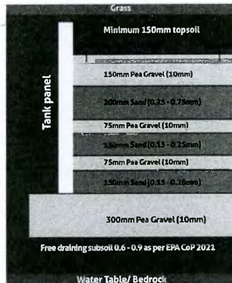
Fig 3.0 Cross section through Sand filter
