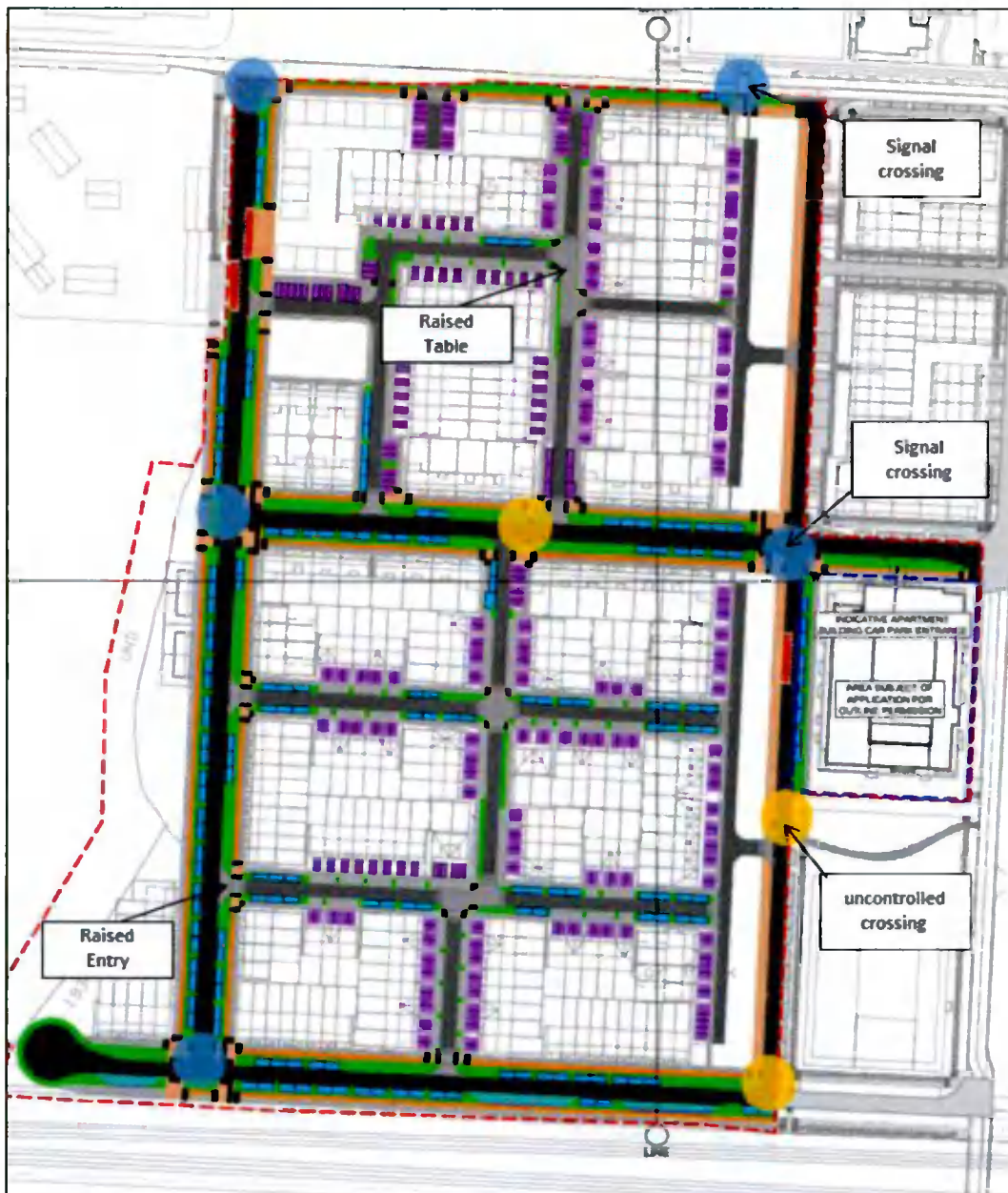
Figure 4-3 - Crossing type and location
