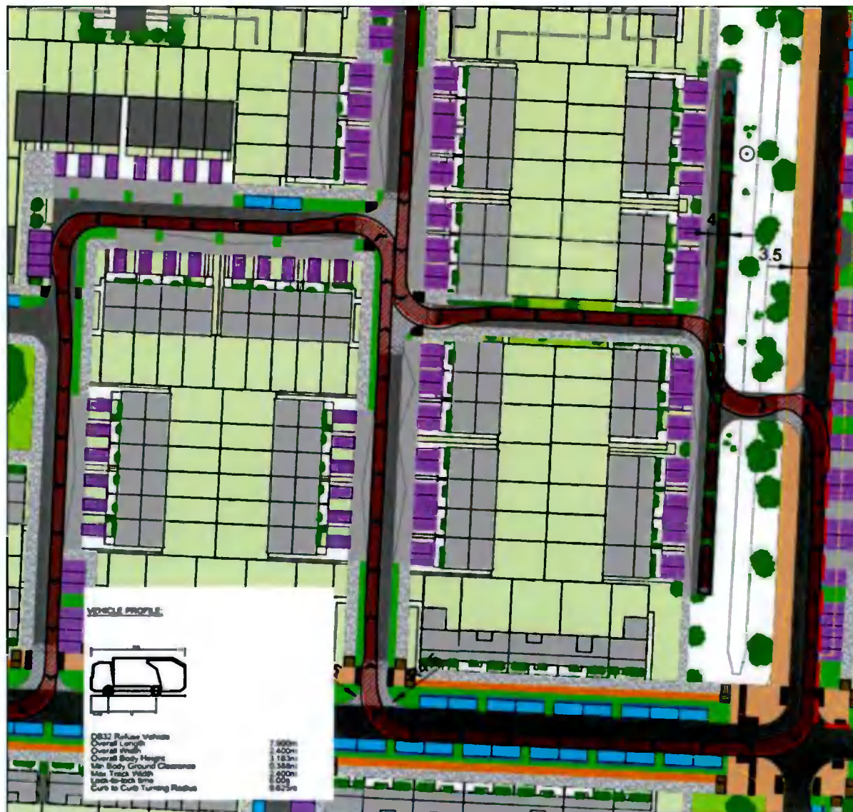
Figure 7-1 - Refuse Vehicle Tracking
