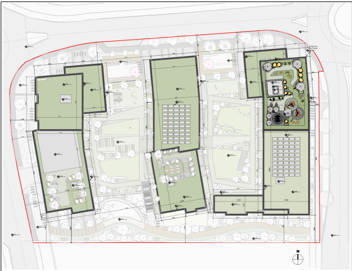
Figure 1: Extract from Drawing No.: 2113 – Drawing BIM Name: PE19150-CWO-ZZ-13-DR-A-2113, a plan view of the of the proposed development showing PV arrays on Block B and Block C.
