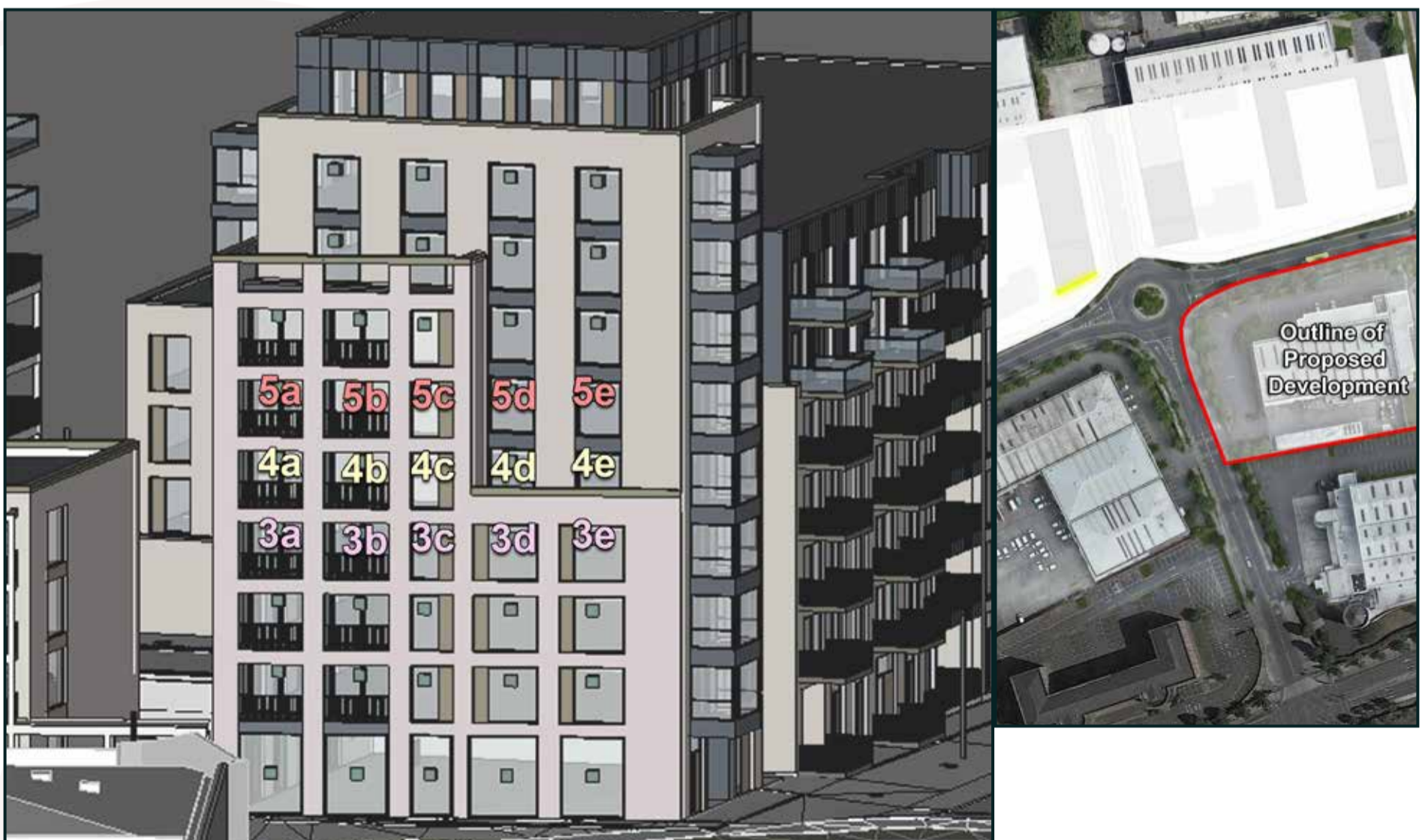
Figure 6.24: Left - Highlighted areas indicate the position of assessed windows., Right - Aerial view of assessed location
