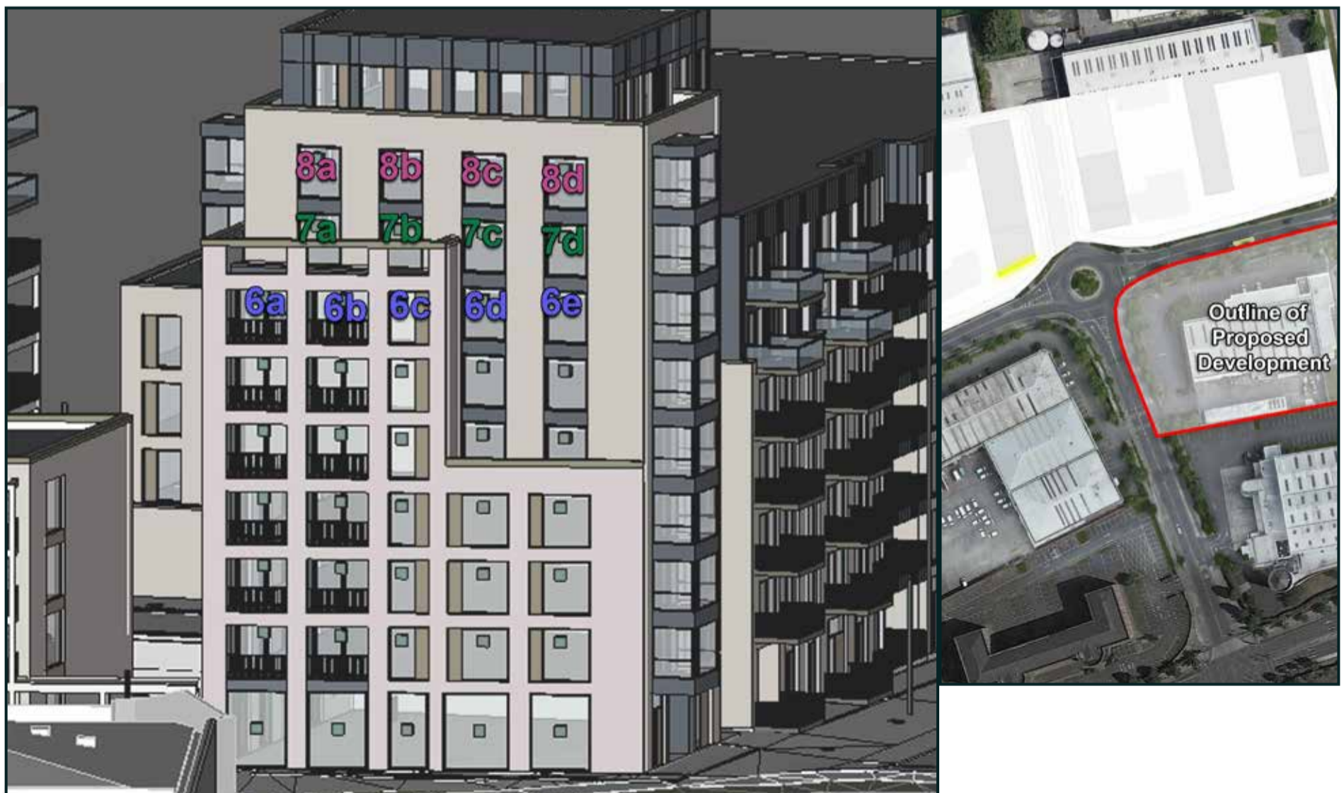
Figure 6.26: Left - Highlighted areas indicate the position of assessed windows., Right - Aerial view of assessed location
