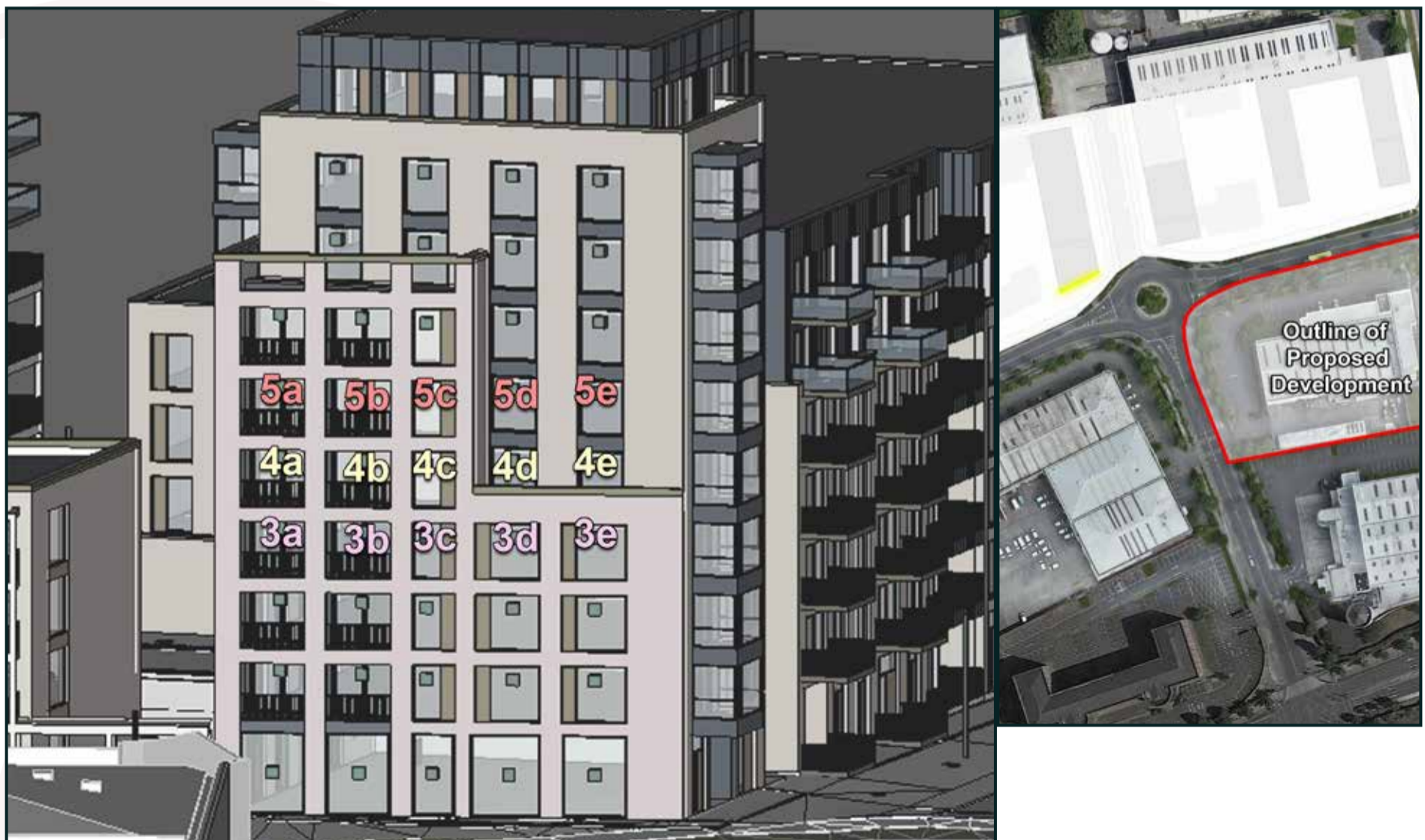
Figure 6.25: Left - Highlighted areas indicate the position of assessed windows., Right - Aerial view of assessed location
