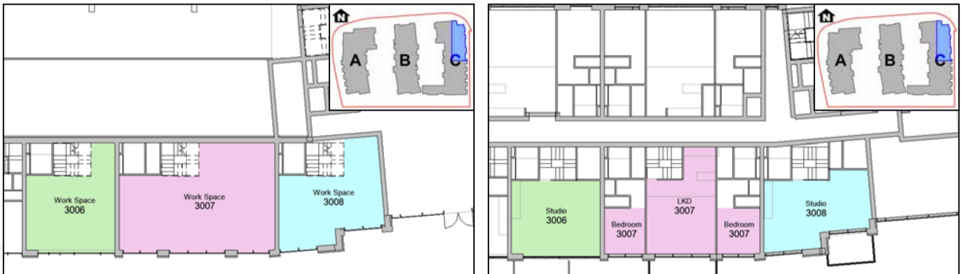
Figure 7.89: Floor plan of assessed rooms with keyplan highlighting the assessed block. Left: Level 00, Right: Level 01
