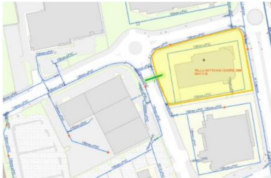
Figure 4 – Proposed Watermain Connection Location (image source: Irish Water Confirmation of Feasibility letter, dated 15/9/2021)
