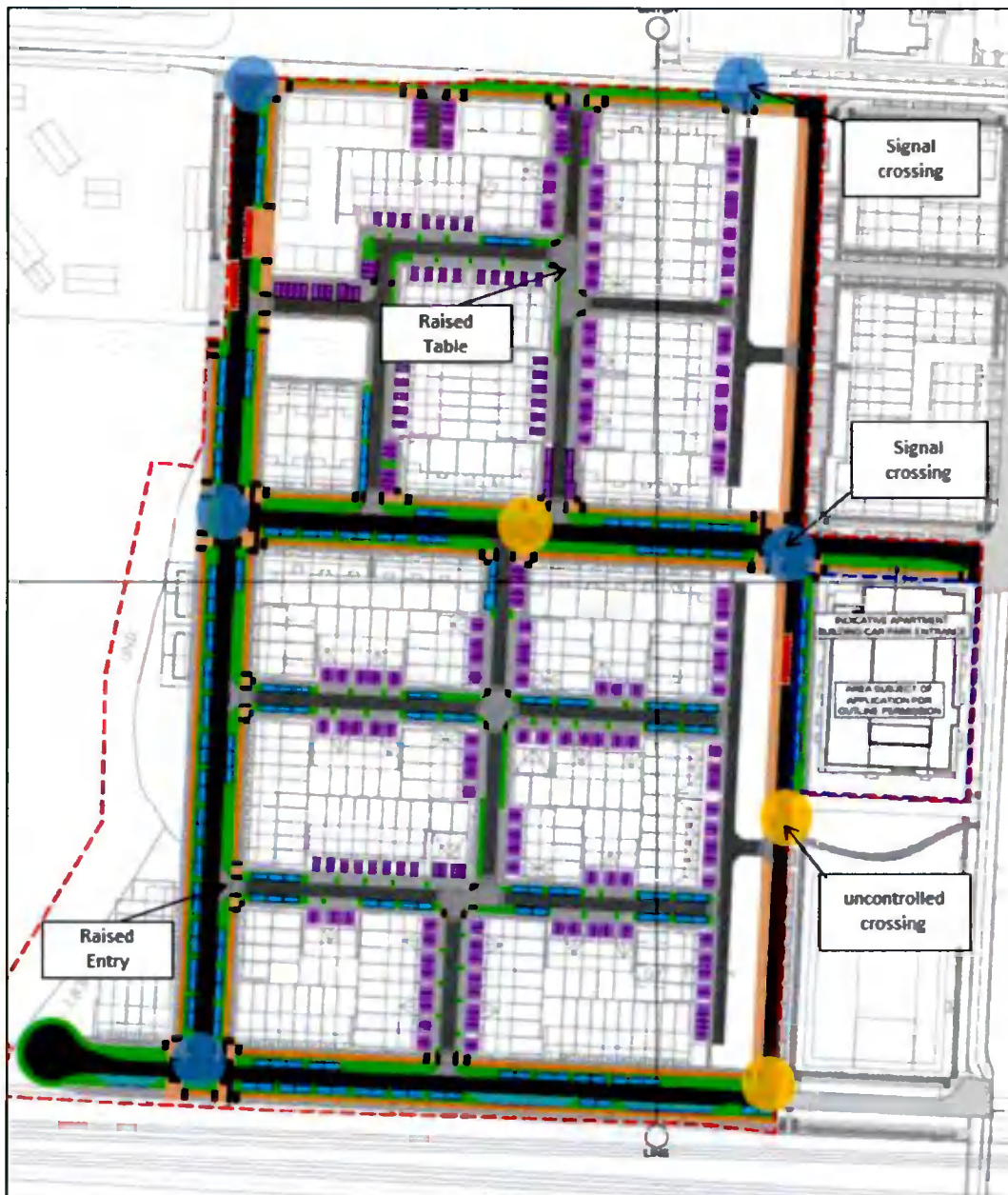
Figure 4-3 - Crossing type and location
