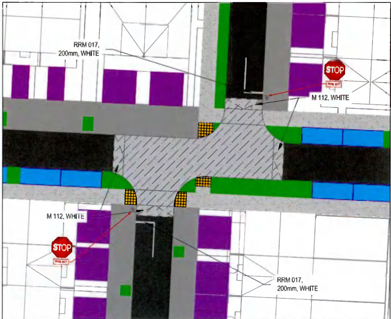
Figure 4-4 - Raised Table Treatment at internal junction
