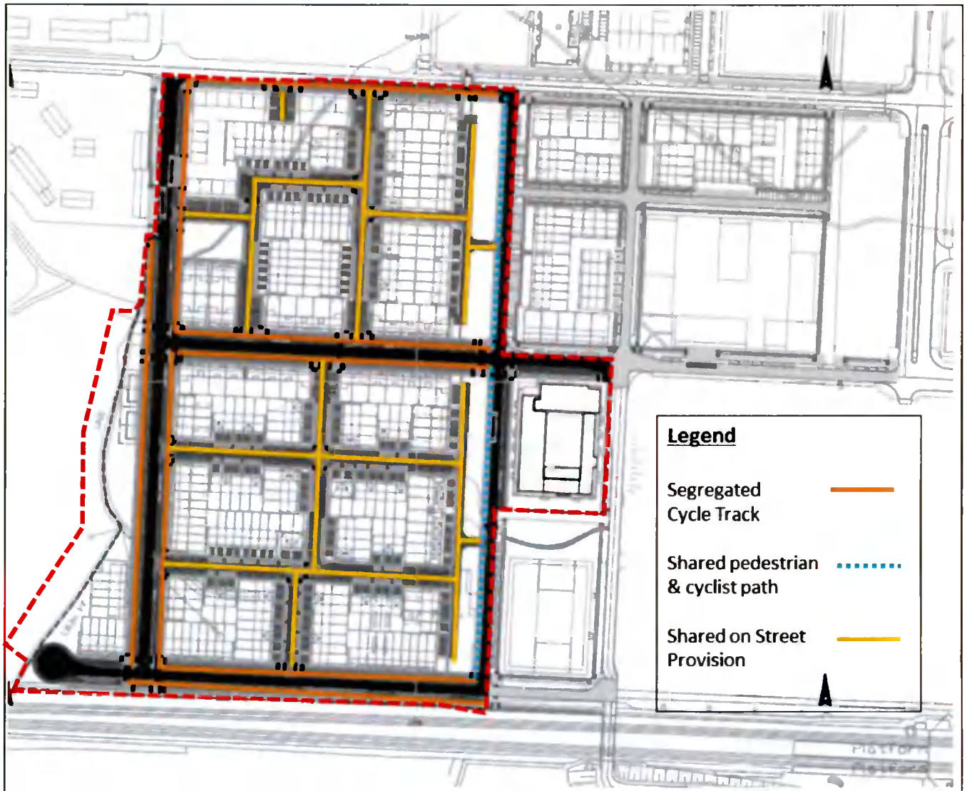
Figure 2-3 - Adamstown Boulevard Phase1 Cyclist Provision
