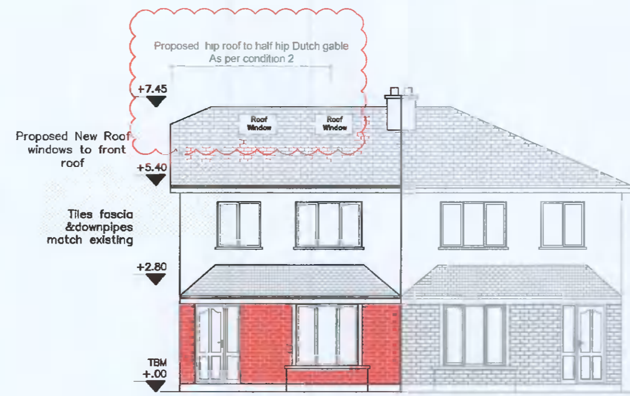
Proposed Front Elevation Scale 1:100
