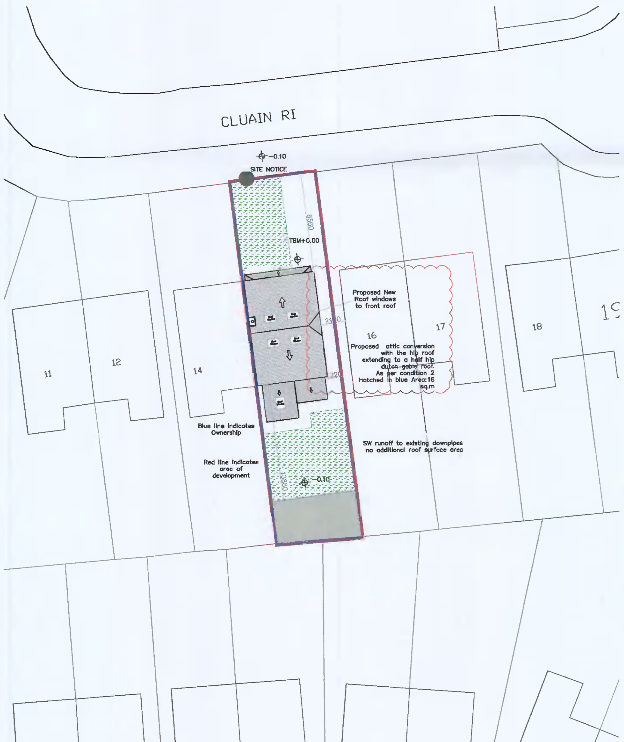
Proposed Site Plan Scale 1:200
