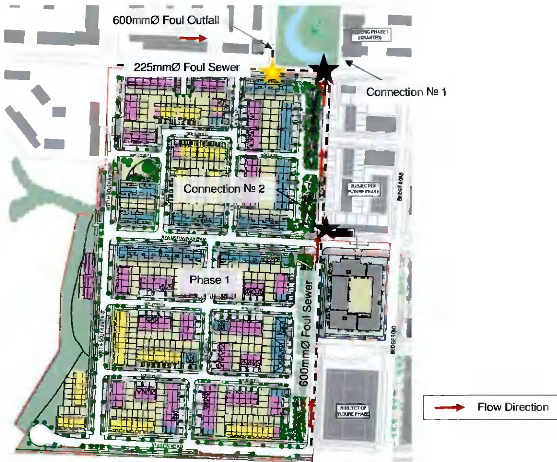
Figure 2-3: Foul Water Sewer Connection Points
