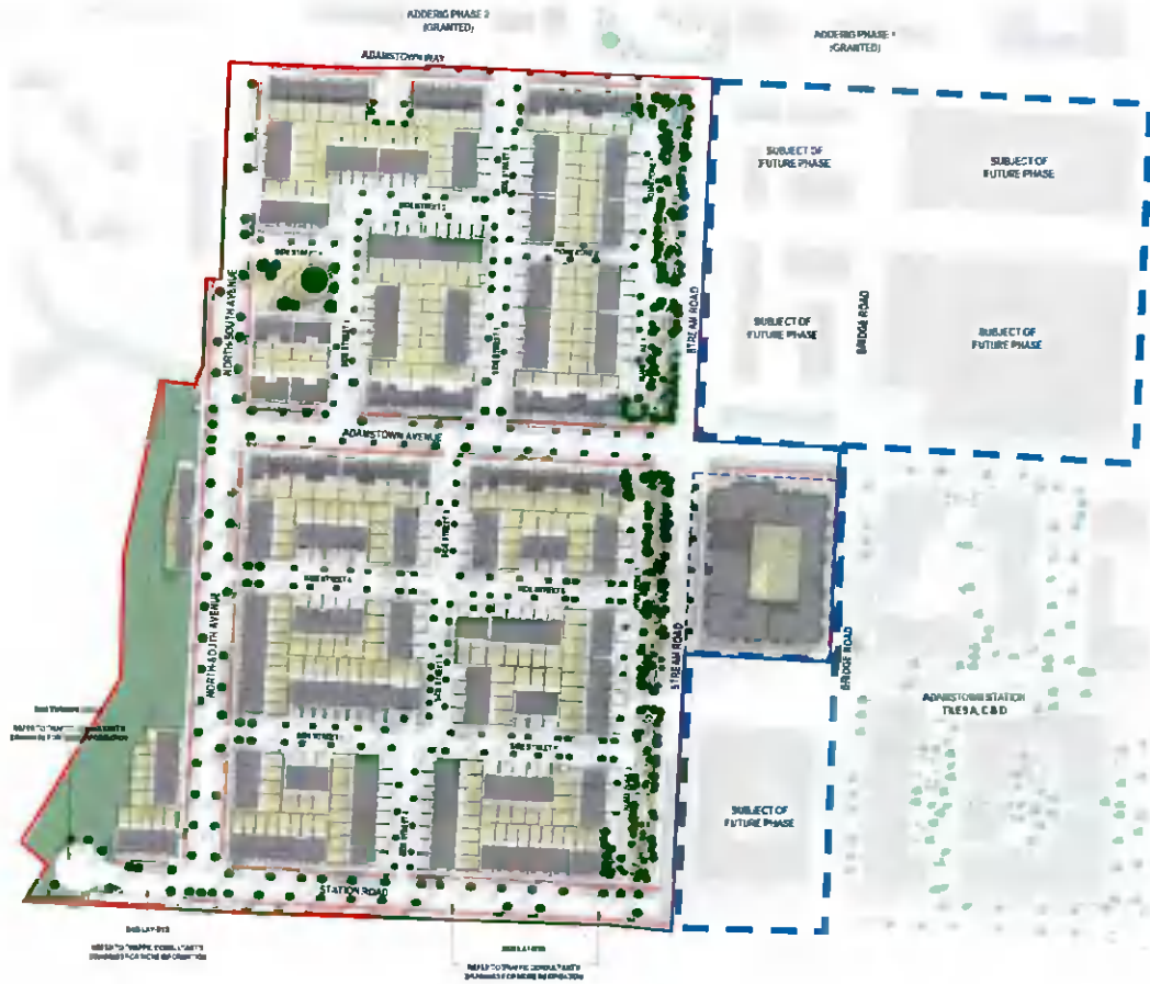
Figure 10: Extract from Overall Masterplan drawing prepared by MDO Architects. Phase 1 site shown within red line, Outline Permission site shaded pink and remainder of site (Phase 2) shown within blue dashed line.
