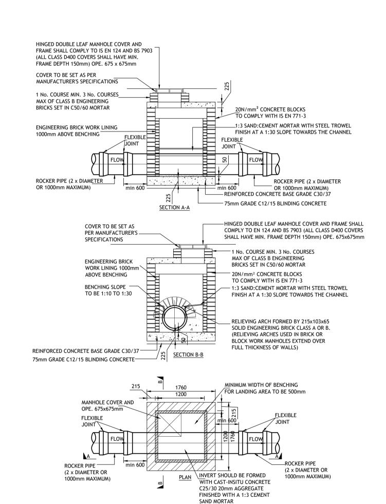
BLOCKWORK MANHOLE (< 450mm DIA.)
