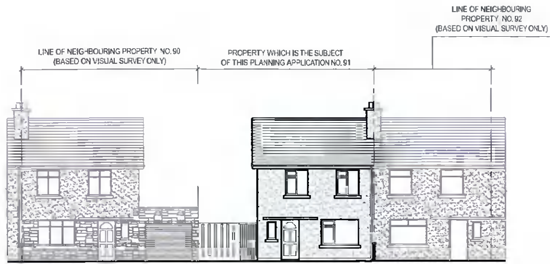
EXISTING SOUTHEAST ELEVATION - FRONT CONTIGUOUS ELEVATIONS SCALE - 1 : 200
