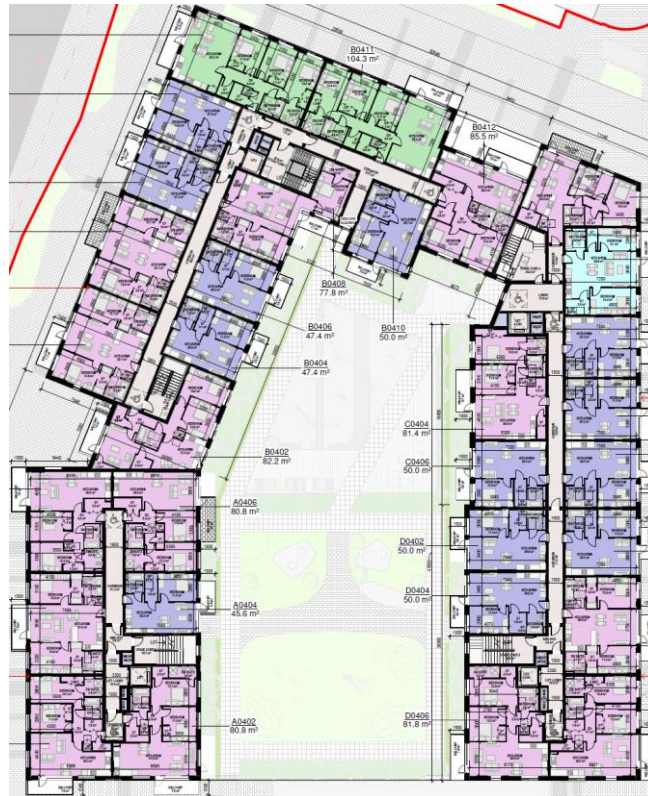
Figure 24.0 Fourth floor plan. We note the provision of 31 no. residential apartments (13 no. one-bedroom apartments, 16 no. two-bedroom apartments and 2 no. three-bedroom apartments) at this level.
