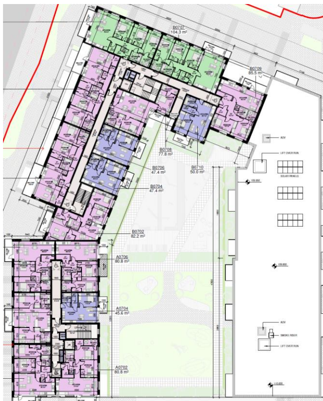
Figure 27.0 Seventh floor plan. We note the provision of 16 no. residential apartments (4 no. one-bedroom apartments, 10 no. two-bedroom apartments and 2 no. three-bedroom apartments) at this level.
