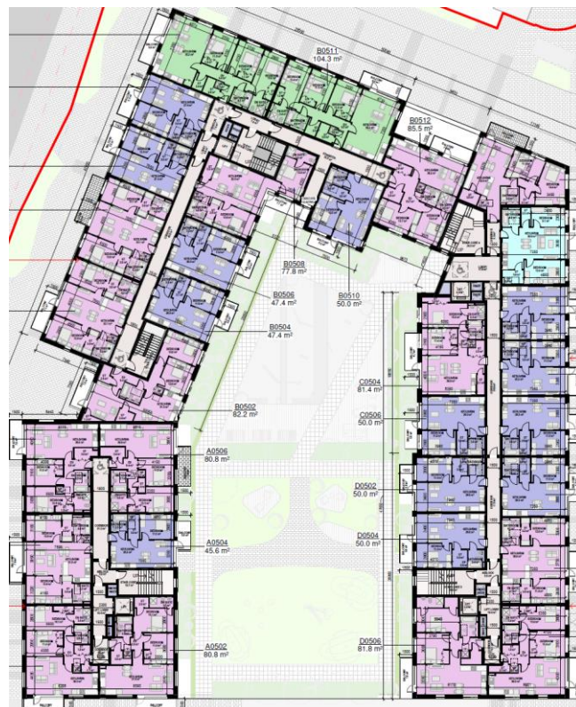
Figure 25.0 Fifth floor plan. We note the provision of 31 no. residential apartments (13 no. one-bedroom apartments, 16 no. two-bedroom apartments and 2 no. three-bedroom apartments) at this level.
