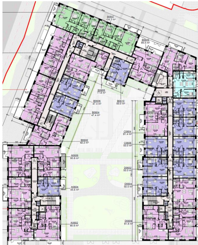
Figure 26.0 Sixth floor plan. We note the provision of 30 no. residential apartments (11 no. one-bedroom apartments, 16 no. two-bedroom apartments and 2 no. three-bedroom apartments) at this level.
