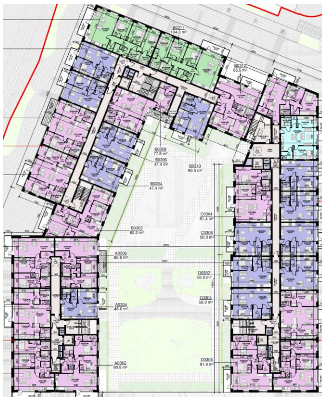
Figure 23.0 Third floor plan. We note the provision of 31 no. residential apartments (13 no. one-bedroom apartments, 16 no. two-bedroom apartments and 2 no. three-bedroom apartments) at this level.
