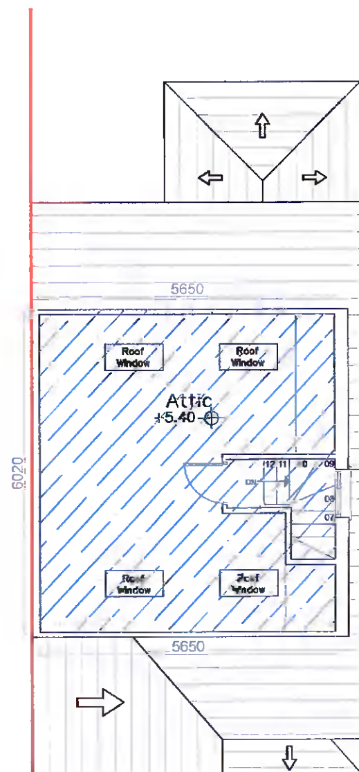
Proposed Attic Floor Plan Scale 1:100 Area 37.65 sq.m
