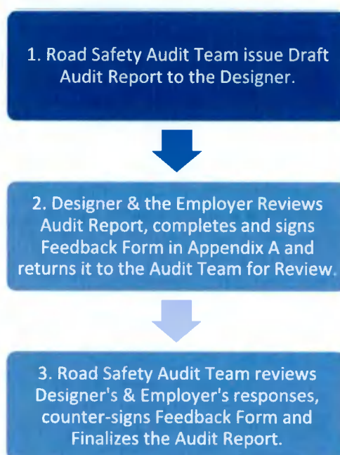
Figure 4.1 – Road Safety Audit Sign-Off and Completion Process
