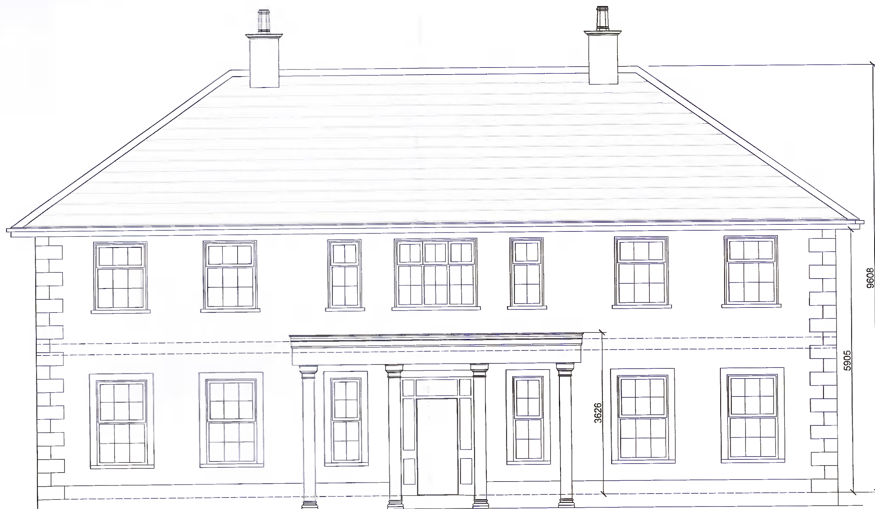
EXISTING WEST (FRONT) ELEVATION 1:50
