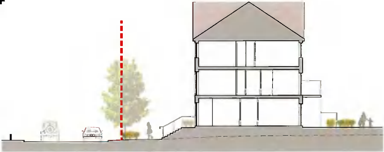
Figure 3.2: Extract from site section showing at-grade footpath and short flight to upper duplexes
