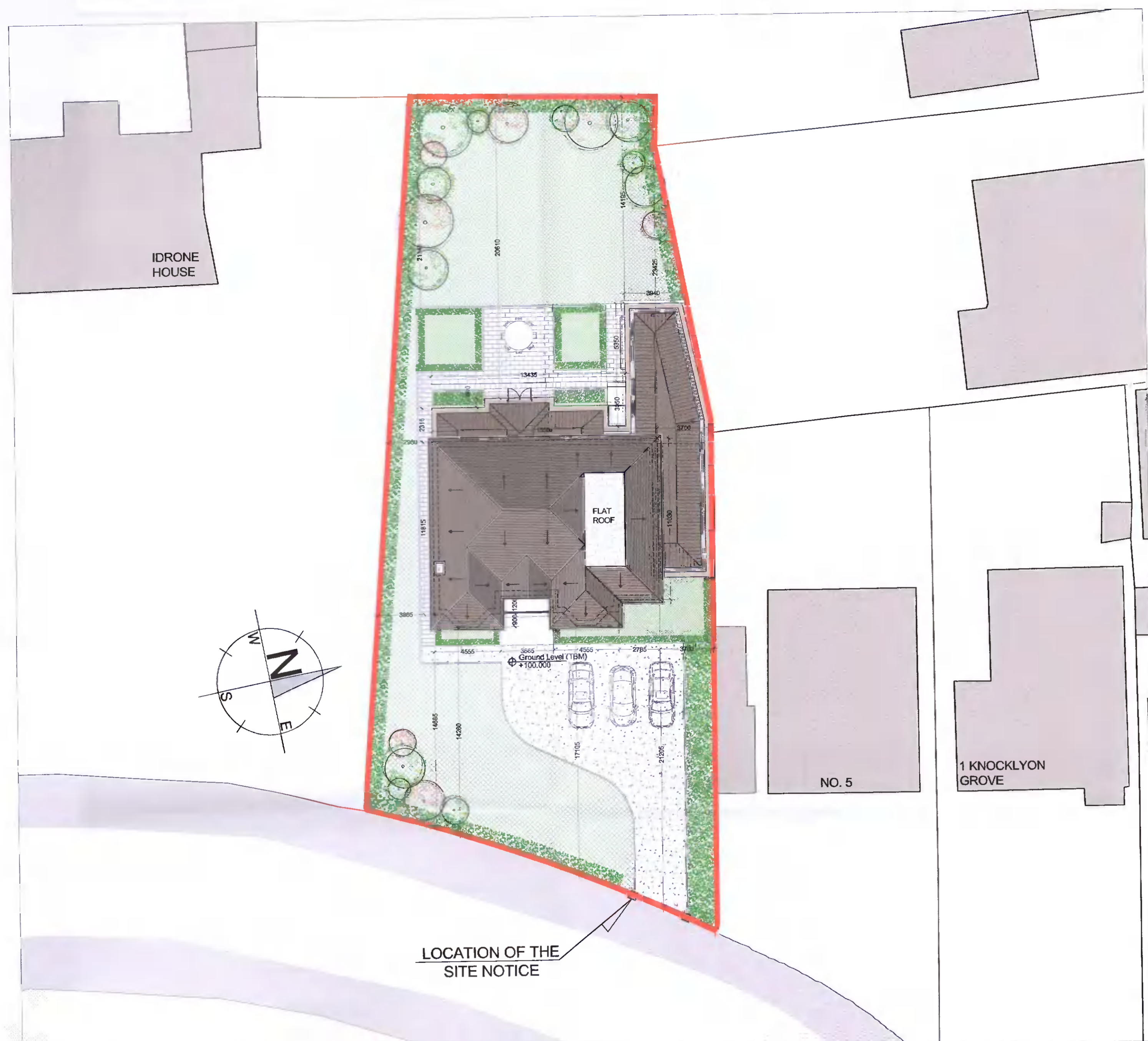
SITE PLAN AND ROOF PLAN AS PREVIOUSLY GRANTED - REG REF. SD205/0286... SCALE 1:200
