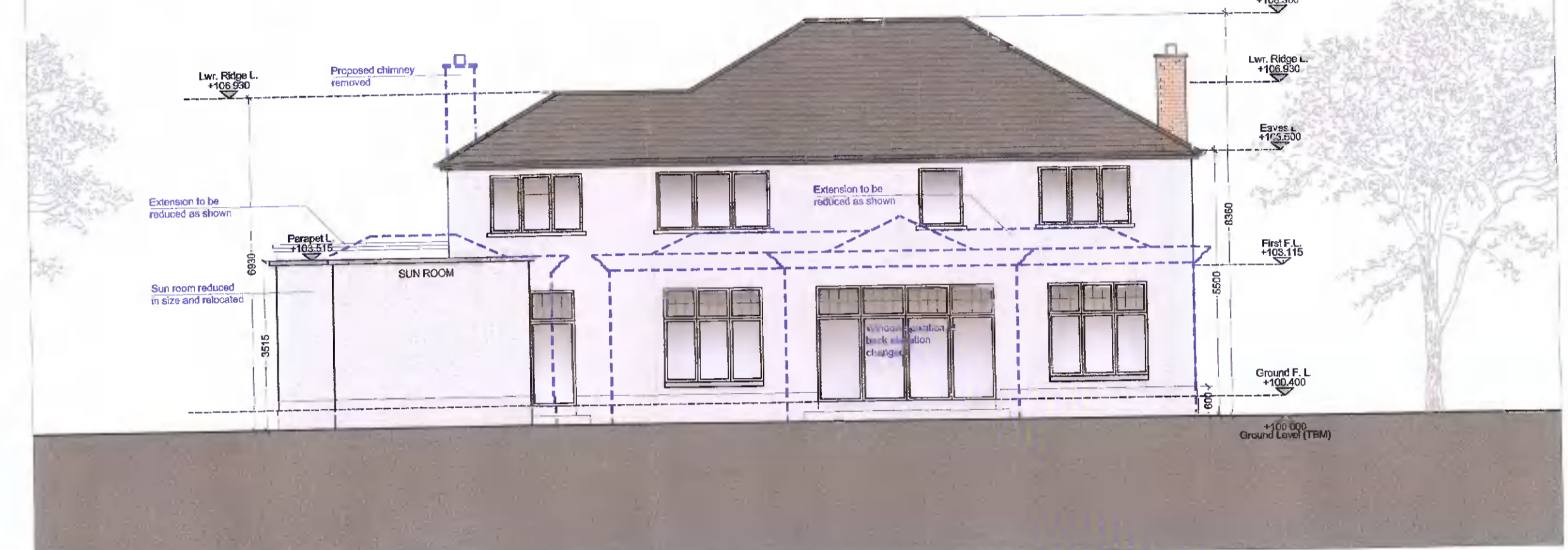
PROPOSED REAR (WEST) ELEVATION ...SCALE...1:100
