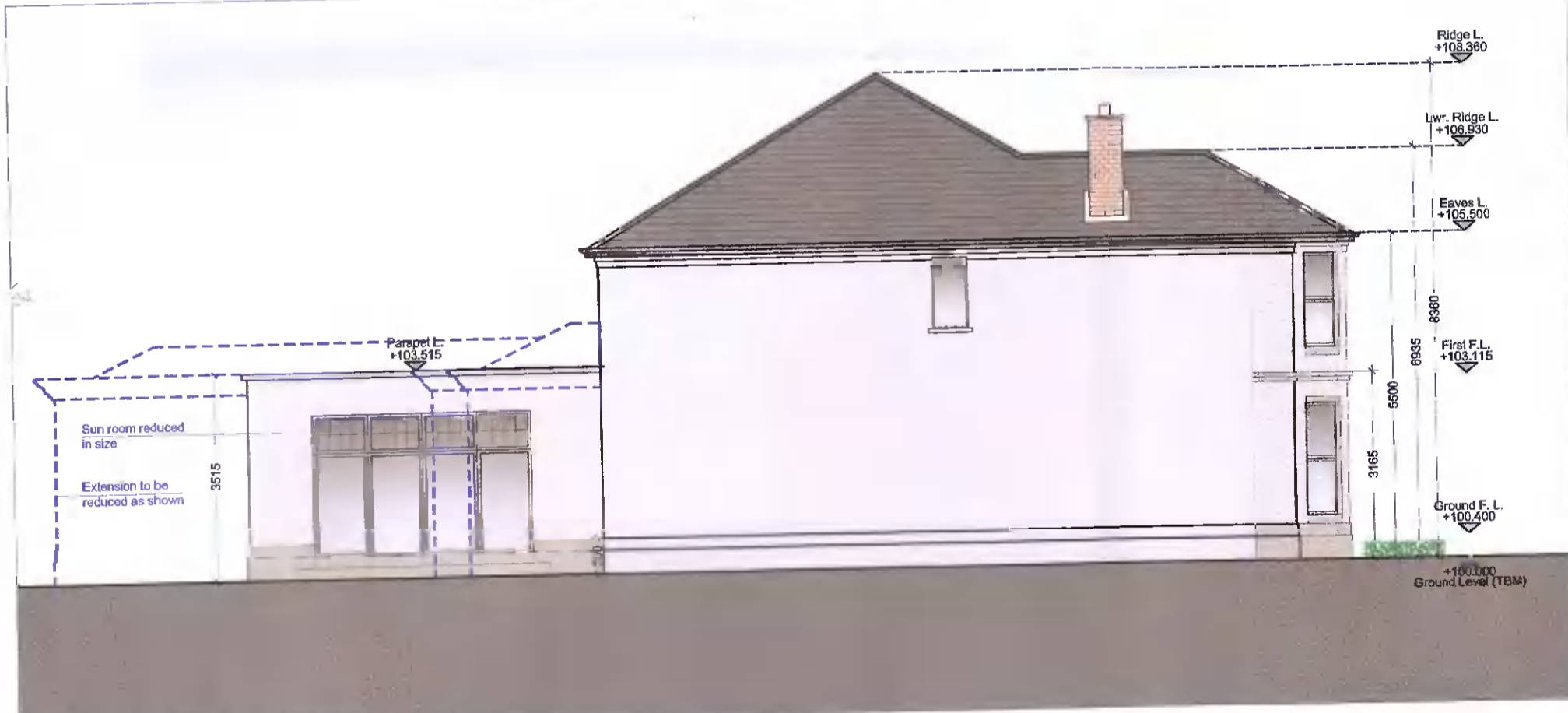
PROPOSED SIDE (SOUTH) ELEVATION ...SCALE...1:100
