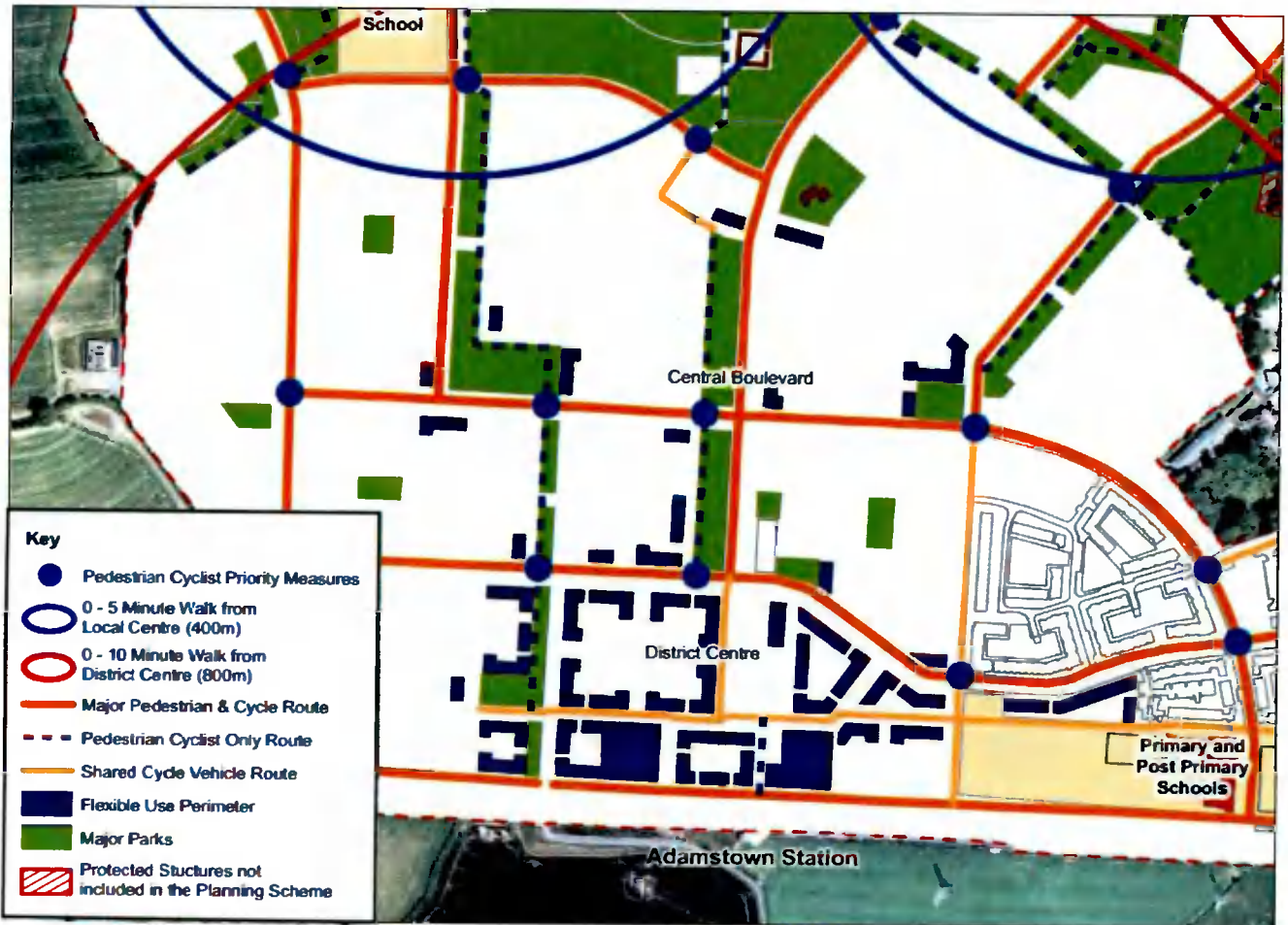
Figure 2-1 - Adamstown SDZ Pedestrian and Cyclist Permeability
