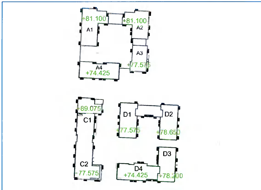
Figure 5: Elevations of Blocks A, C and D
