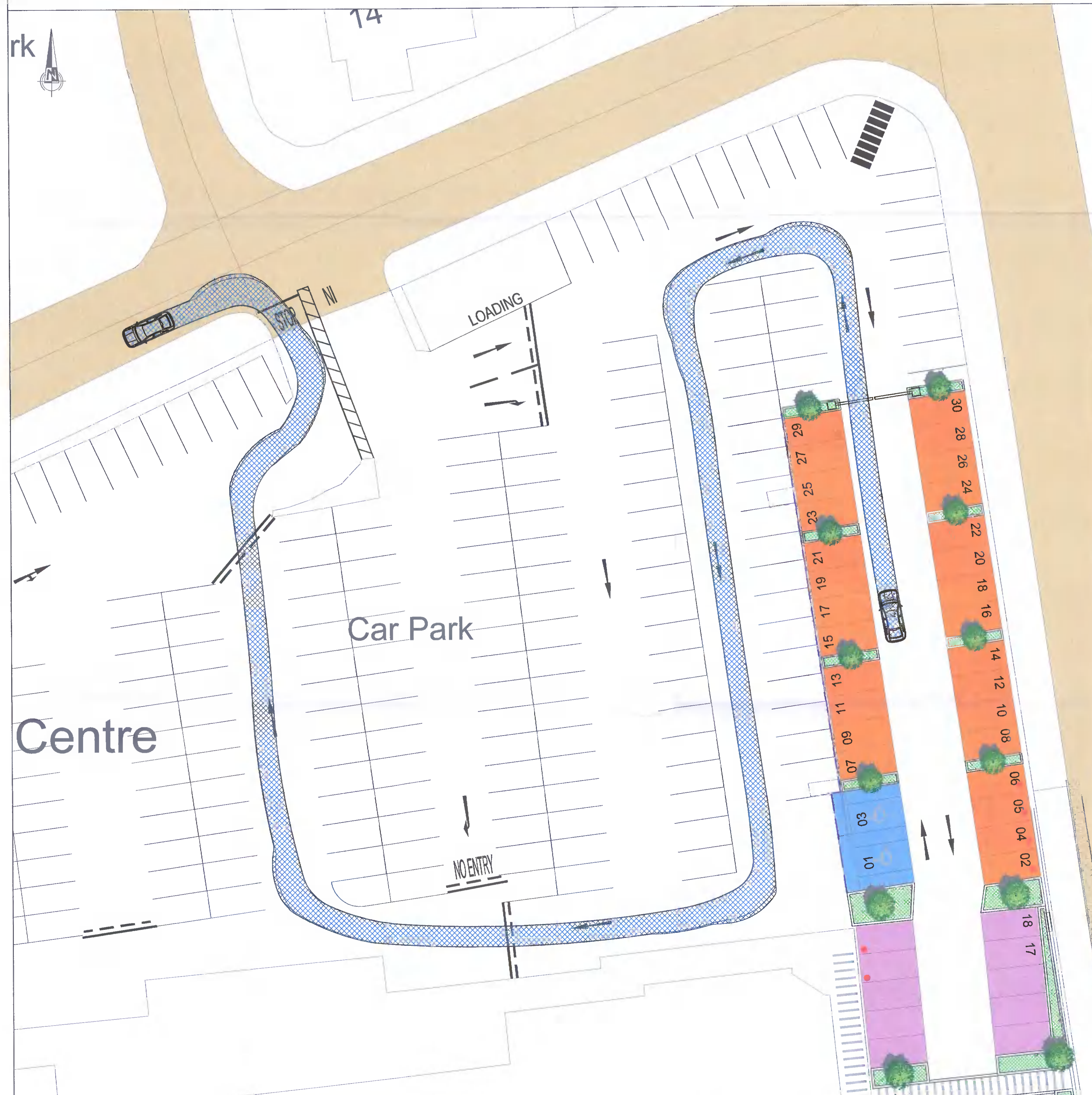
AUTOTRACK OF A LARGE SALOON CAR EXITING THE SHOPPING CENTRE CAR PARK
