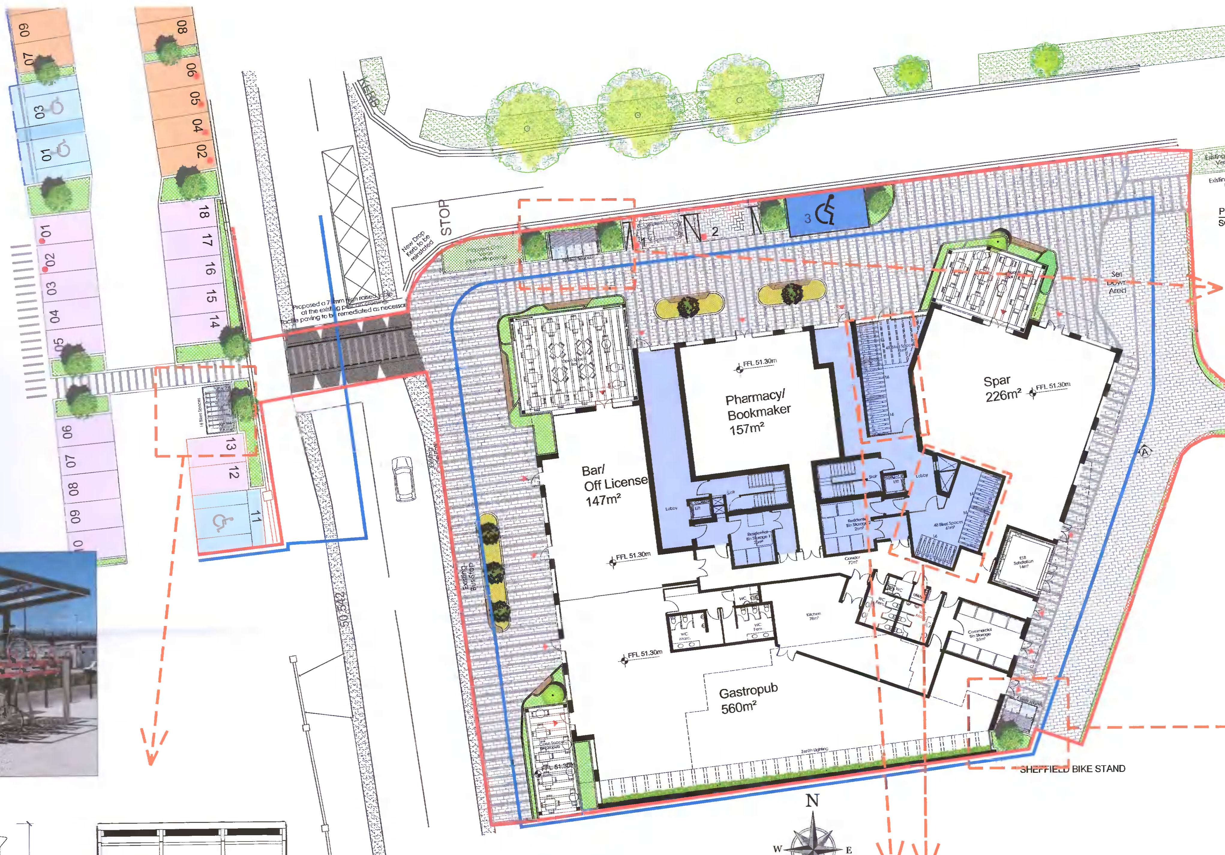
PROPOSED SITE LAYOUT - GROUND FLOOR PLAN SCALE 1:200
