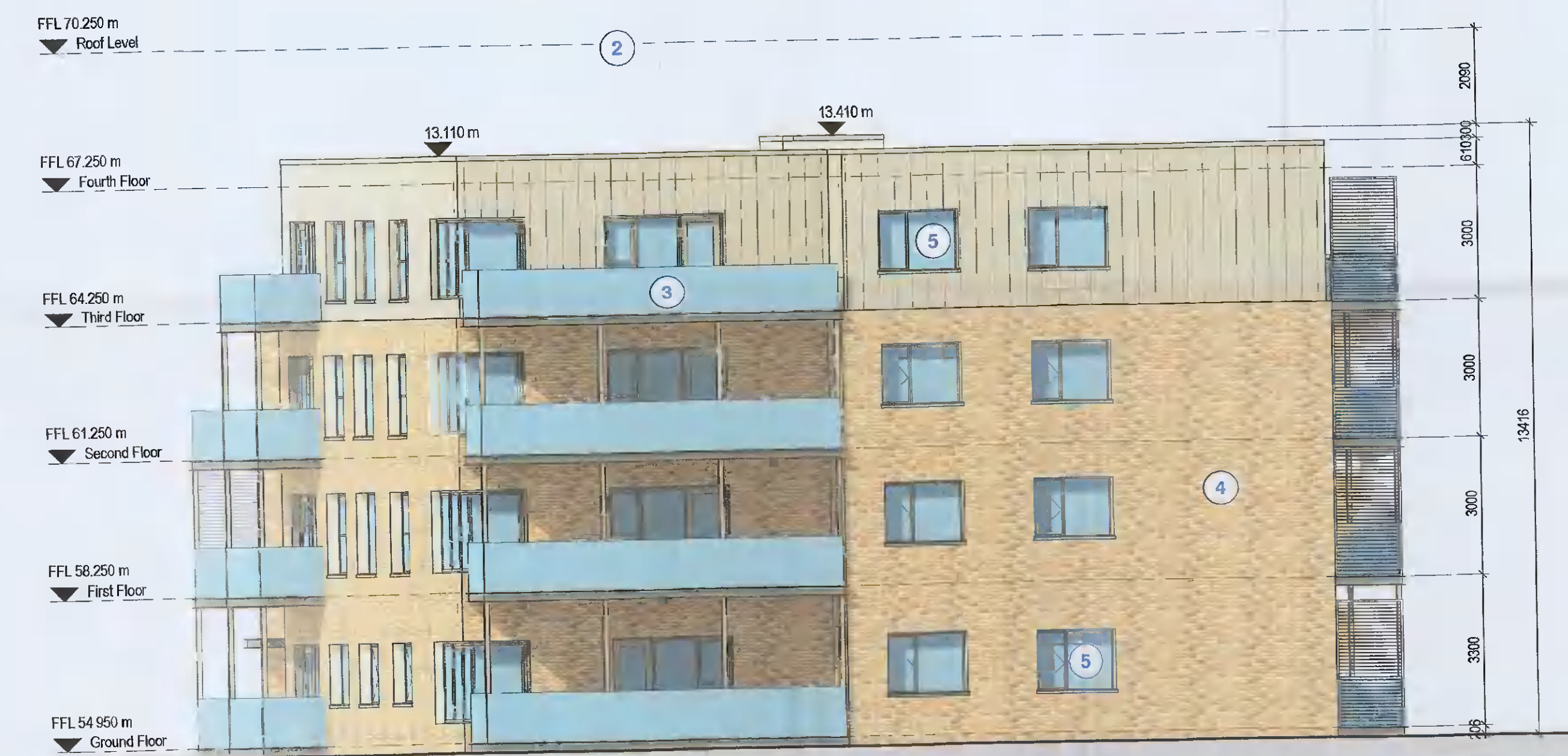
BLOCK 3 EAST ELEVATION FACING BLOCK 2 1 : 100
