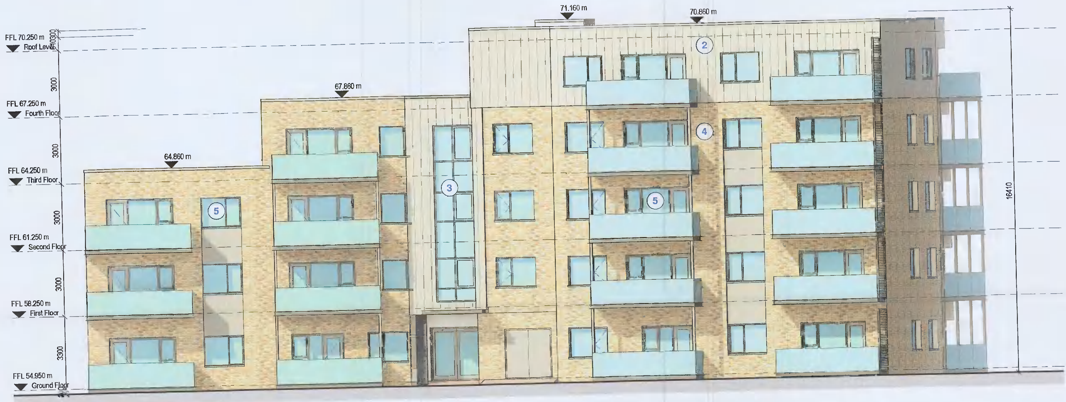
BLOCK 2 WEST ELEVATION FACING ACCESS ROAD 1 : 100
