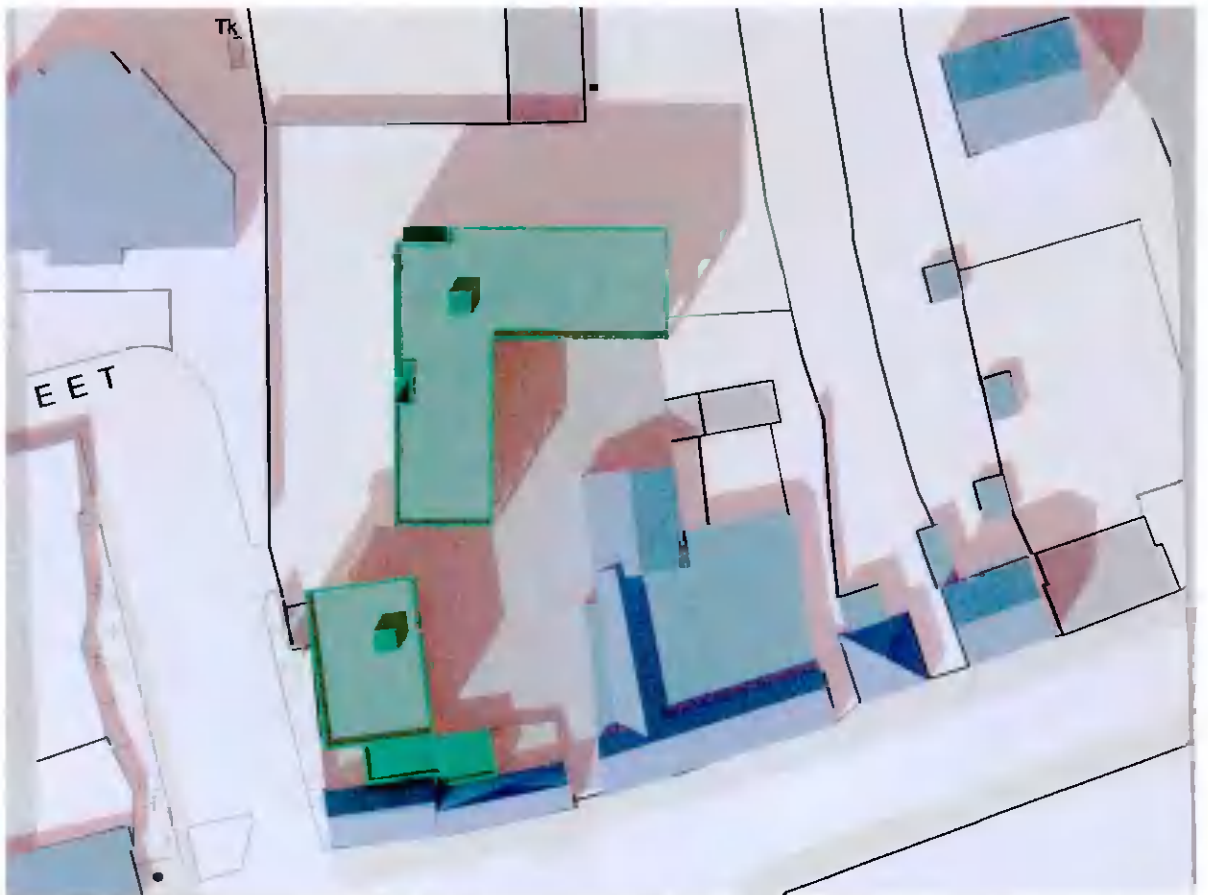
Figure 21: Shadow diagrams 21 September 15:00 GMT +1 (DST)
