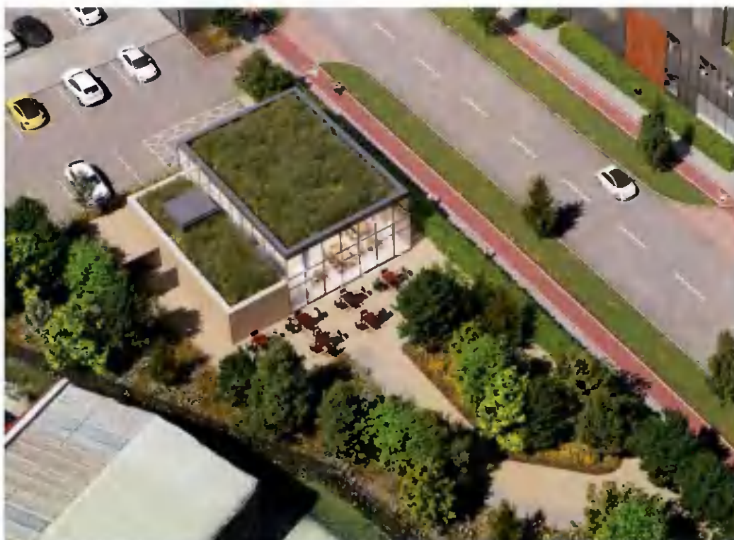
Extract from Aerial CGI View by others showing café unit off Calmount Road, with intensive green (brown) roofs and SuDS Garden with Bioretention areas and swales to the road verges. (Please note this is an Artists' Impression; planting proposals are not accurate as per the species proposed, but show an overall impression in spatial and visual terms)
