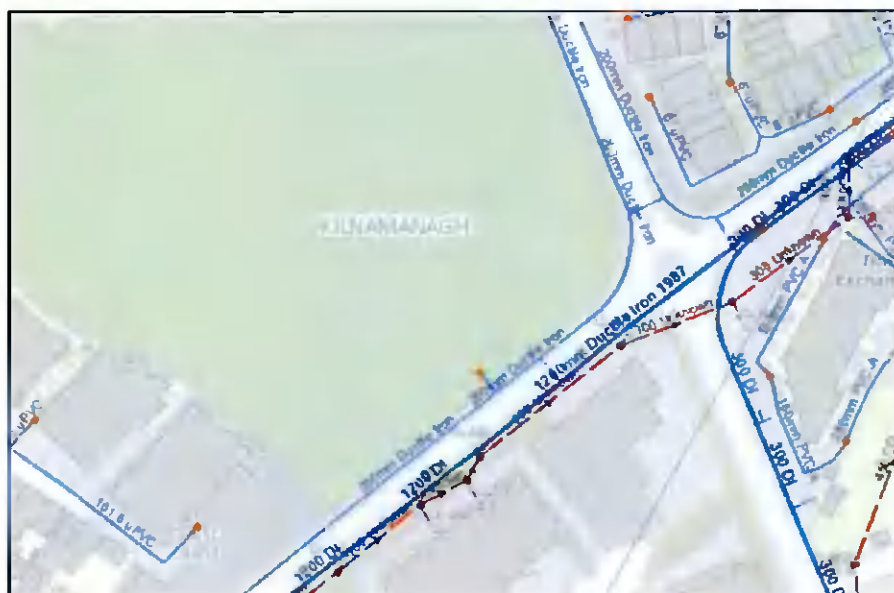
Figure 2-1 Existing Foul Water Sewer Infrastructure
