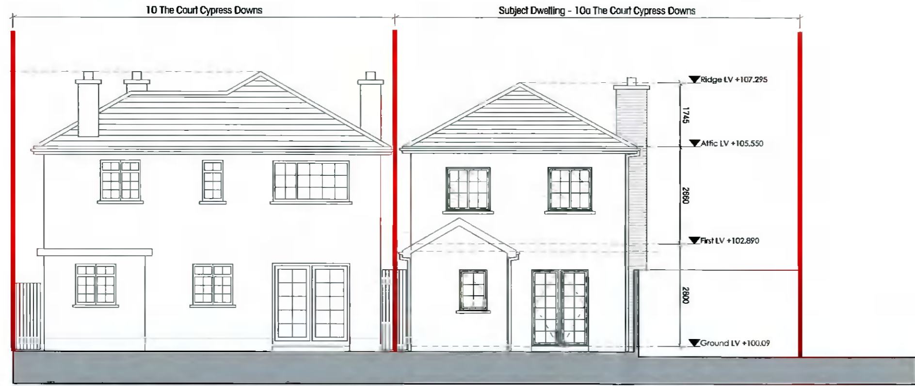
2. EXISTING CONTIGUOUS REAR (EAST) ELEVATION
