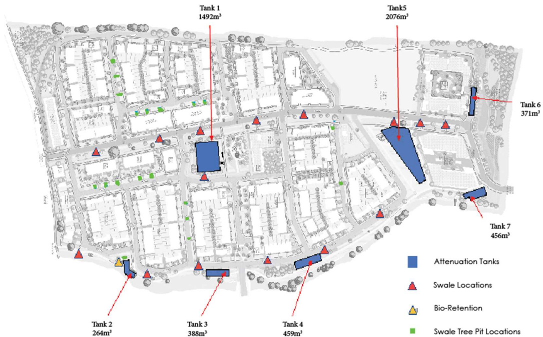
Fig. 13.5 – Sustainable Drainage Systems
