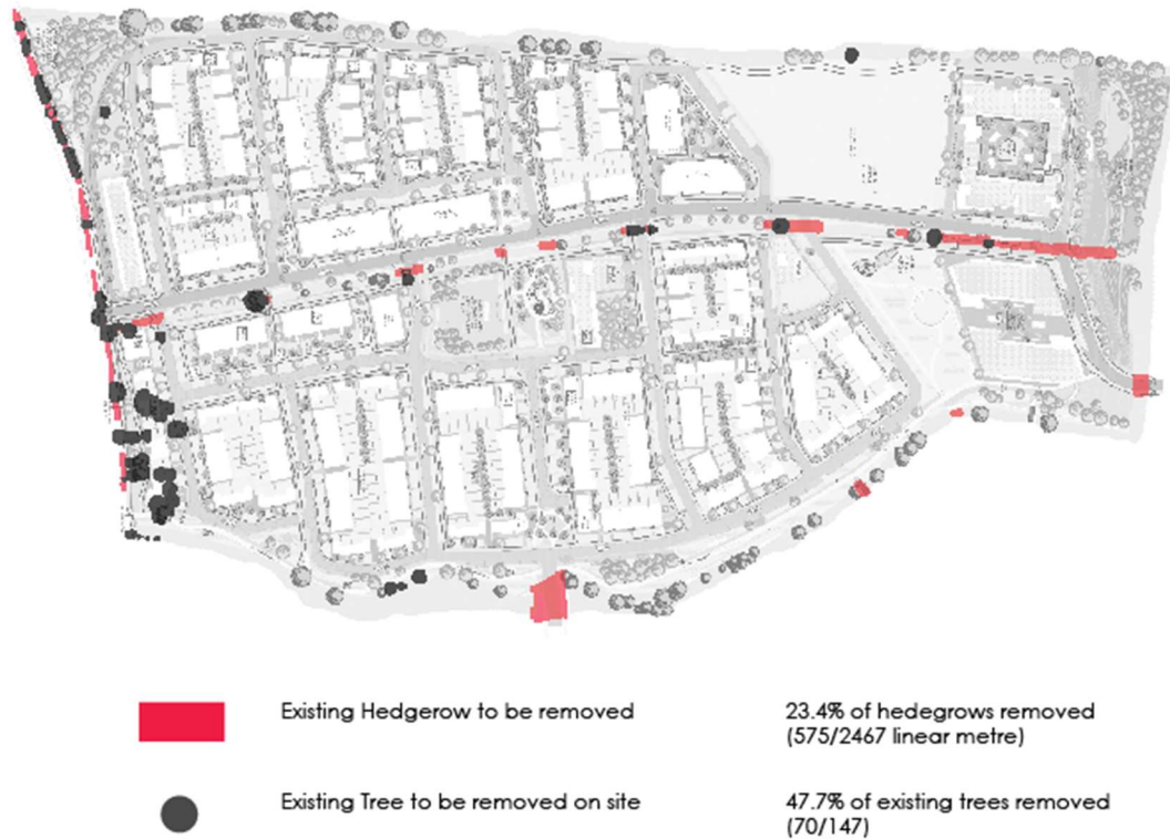
Fig. 13.17 – Tree & Hedgerow Removal
