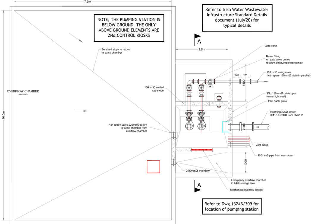
Below Ground Pump Station Plan
