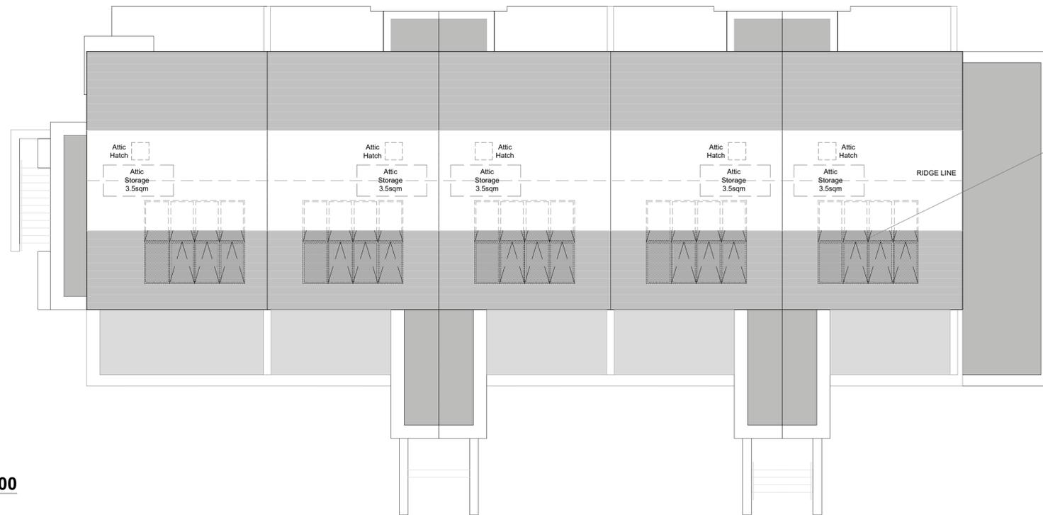
Indicative solar panel position, final solar panel quantity & position subject to detailed design, on duplex block orientation and final BER requirement at the time of publication. The solar panels shown are a provisional option to satisfy renewable energy requirements of building regs part L. Solar panels may be omitted in favour of alternative renewable energy source.
