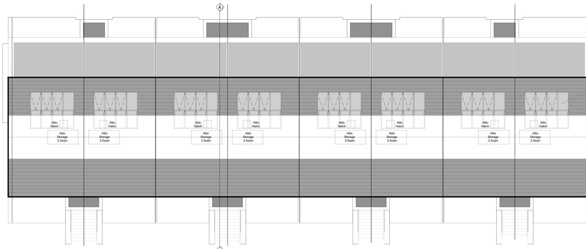
Indicative solar panel position, final solar panel quantity & position subject to detailed design, on duplex block orientation and final BER requirement at the time of publication. The solar panels shown are a provisional option to satisfy renewable energy requirements of building regs part L. Solar panels may be omitted in favour of alternative renewable energy source.
