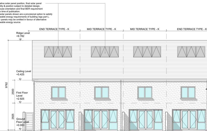
**REAR ELEVATION (Terraced Type K)**
