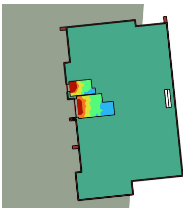
Figure 32: Block B - All floors false colour plans of ADF. Scale 0 - 5%
