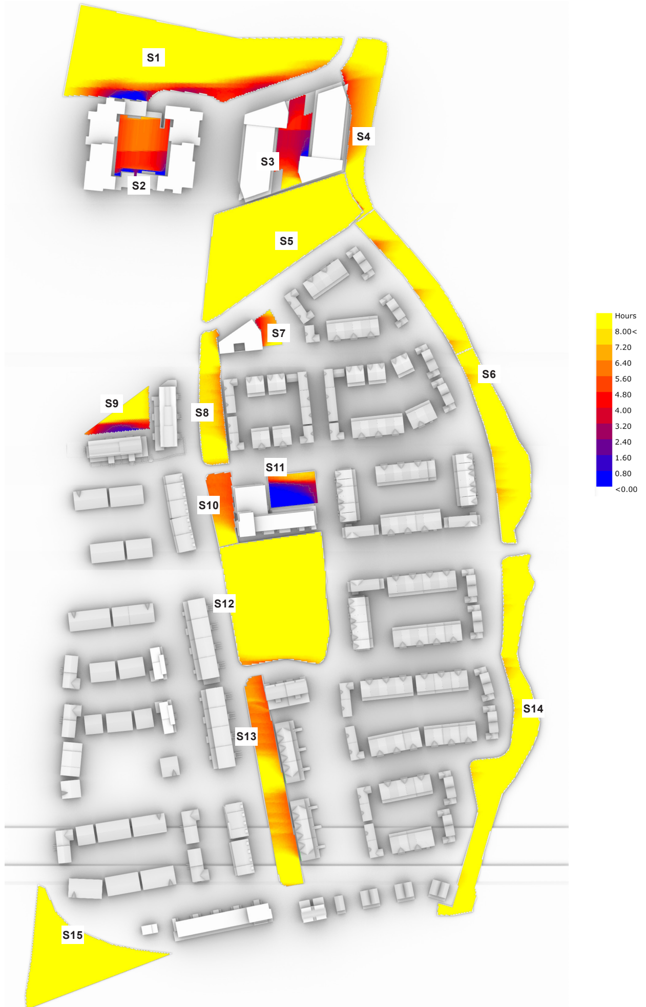
Figure 8: Radiation map of amenity areas, showing available sunlight on 21st March. The scale represents the percentage of daylight received from 0 - 8 hrs.
