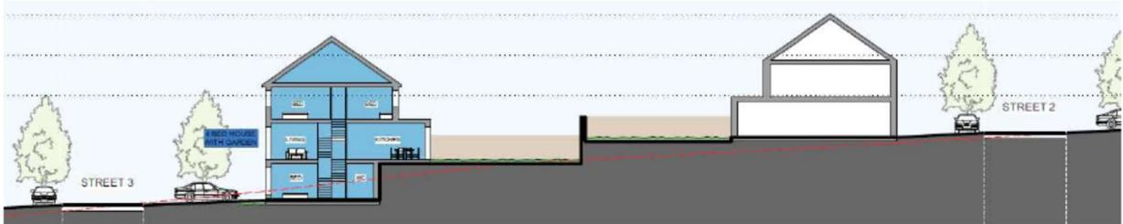
Fig. 15 – Schematic drawing of split level house typology to minimize step in level between adjacent rear gardens
