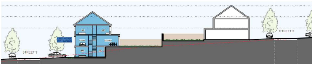
Fig. 10 – Schematic drawing of split level house typology to minimize step in level between adjacent rear gardens
