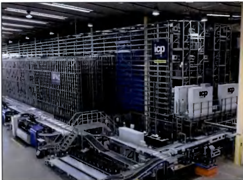
Figure 3.1: The Main 'Cubi Shuttle Block' that Protrudes from the First Floor Mezzanine Through the Mezzanine Floor Above. Source: Uniphar Image
