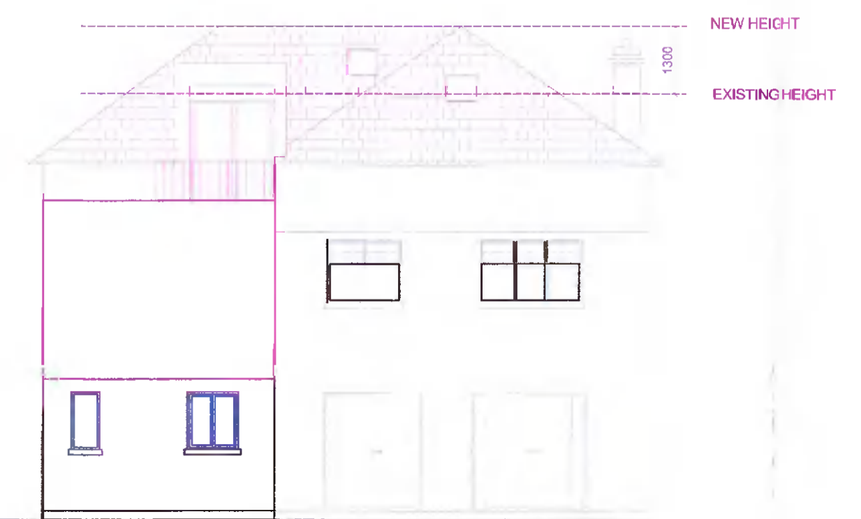
PROPOSED REAR ELEVATION SCALE 1:100
