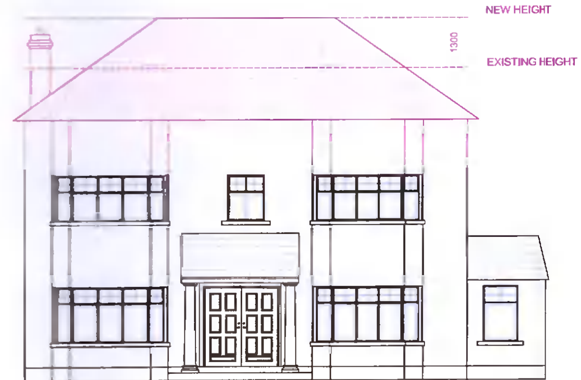
PROPOSED FRONT ELEVATION SCALE 1:100
