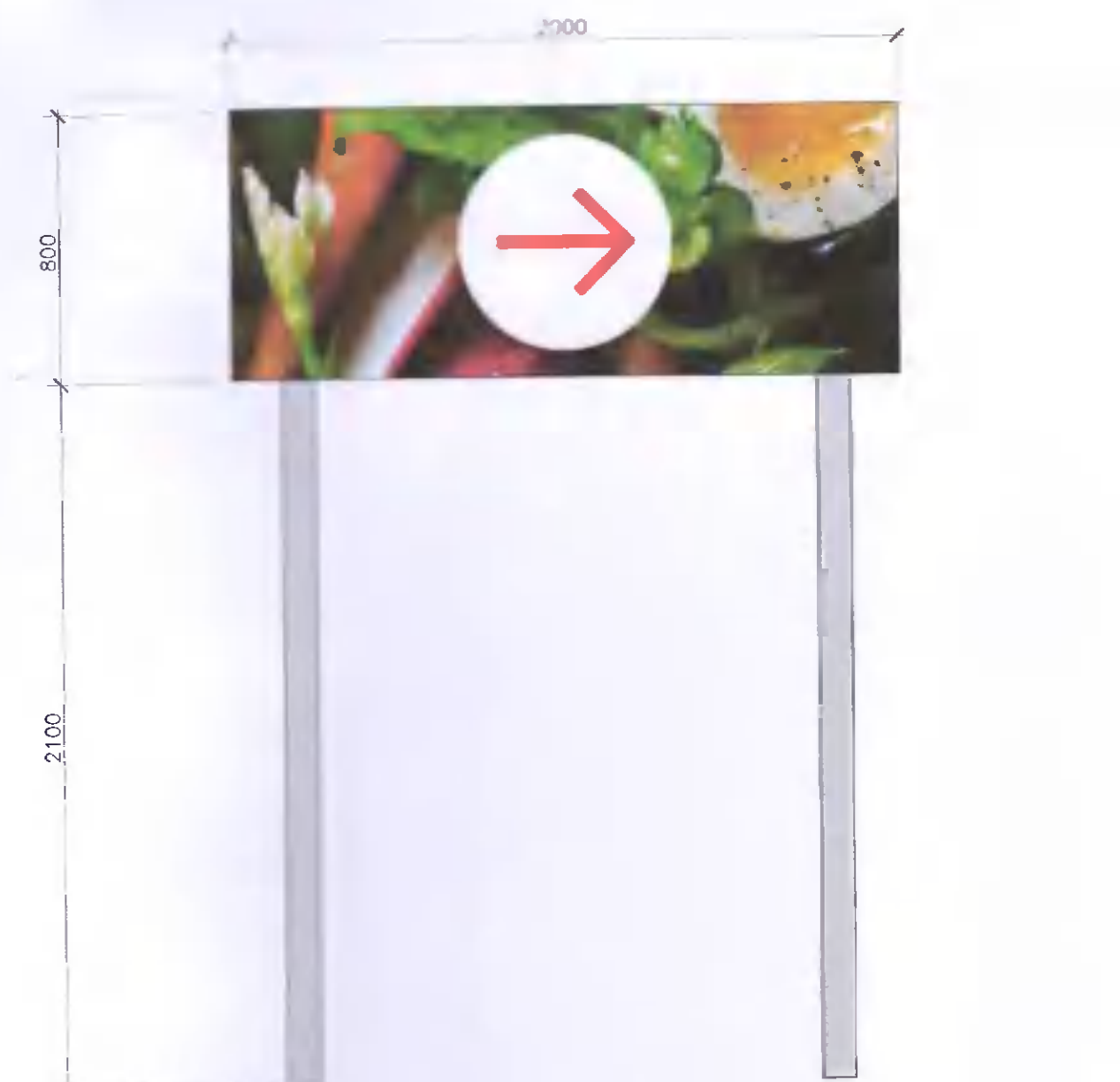
INTERIOR VIEW SIGNAGE – SIDE ELEVATION SCALE 1:20
