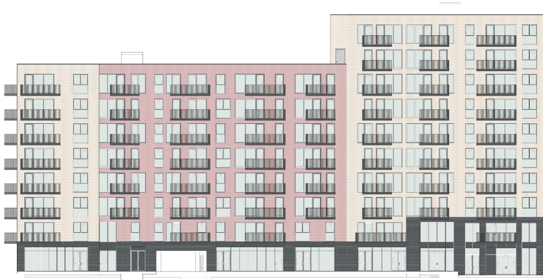
Figure 5-11. Glazing to facade ratio of the east elevation of Block A (C + W O'Brien Architects).
