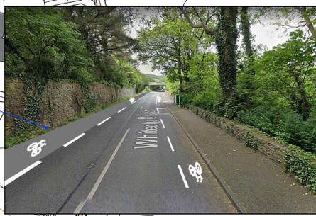
IMAGE ILLUSTRATING 'ADVISORY CYCLE LANE' MARKINGS ON WHITECHURCH ROAD IN LINE WITH THE NATIONAL CYCLE MANUAL
