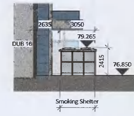
2 03023 Smoking Shelter - East Elevation 1 : 200
