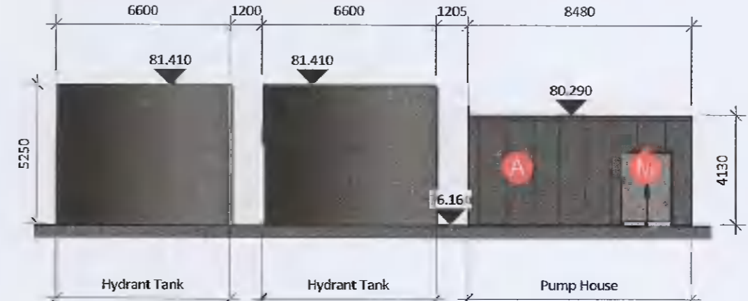
13 03023 Pump House - North Elevation 1 : 200
