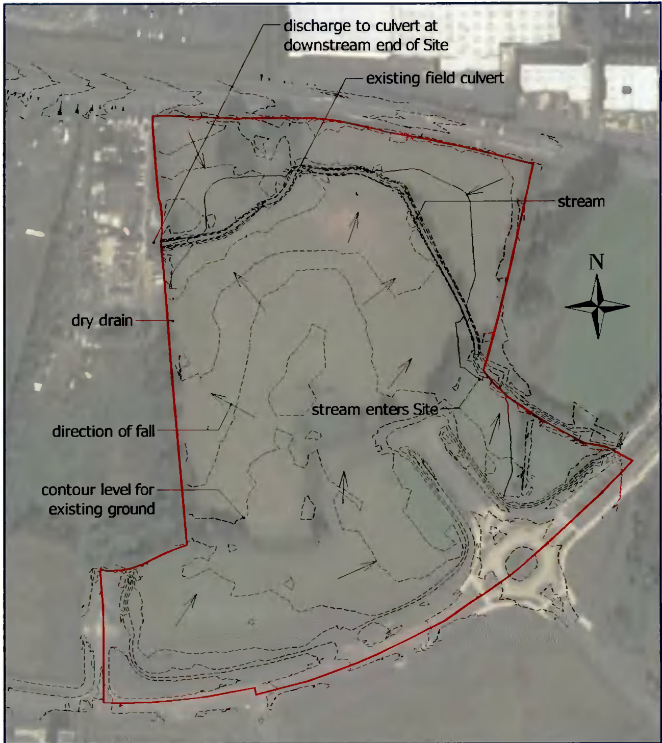
Figure 3-2 Site Topography / Main Drainage Features
