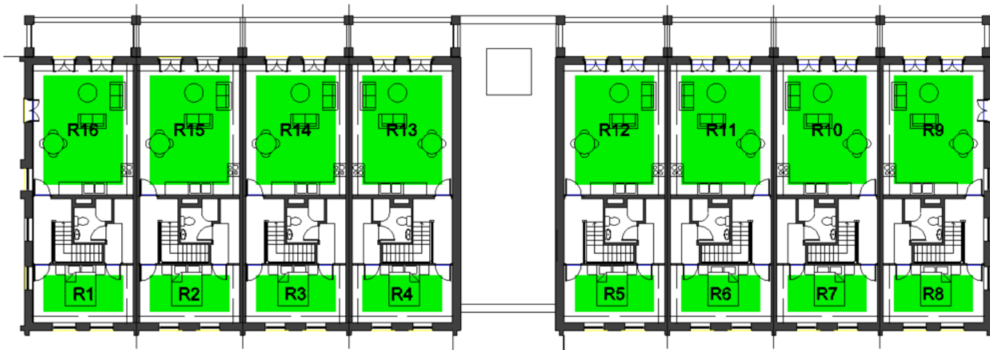
Figure 37: Block E Third Floor sDA Pass/Fail Contour
