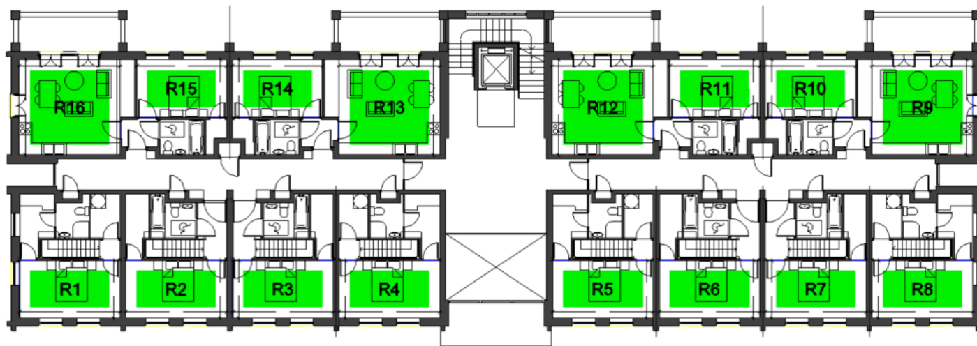
Figure 35: Block E First Floor sDA Pass/Fail Contours
