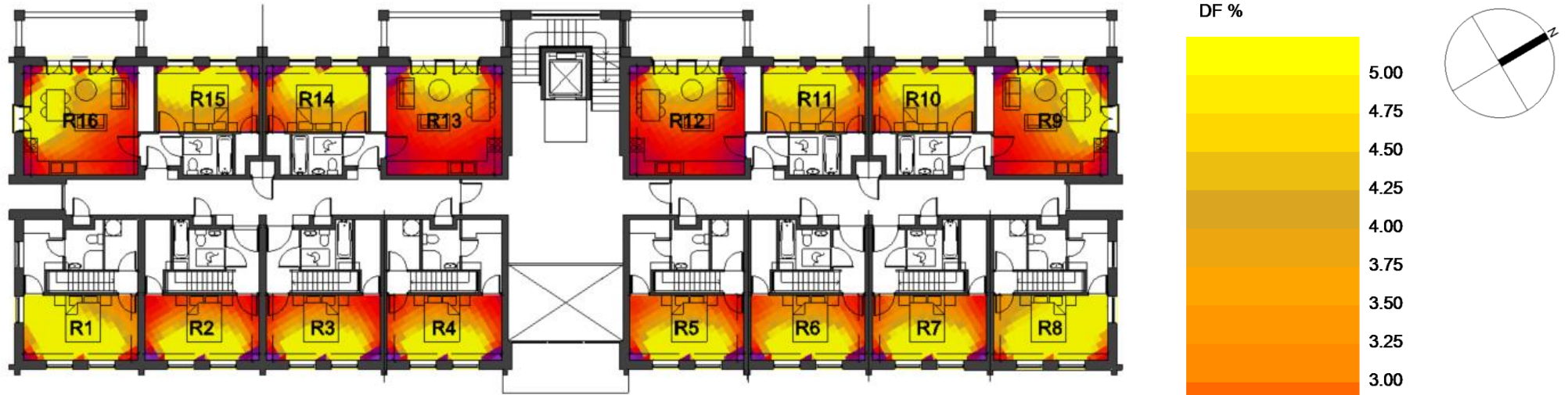
Figure 20: Block E First Floor DF Contours
