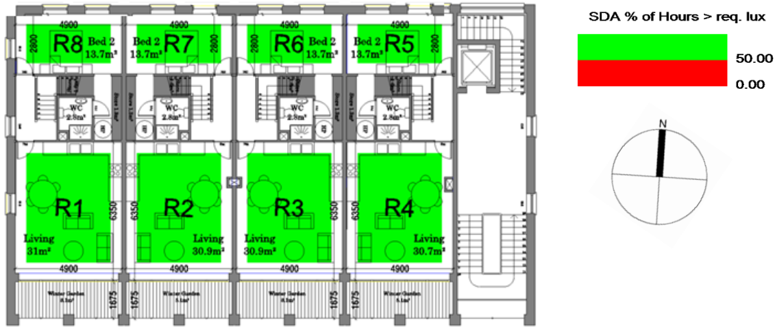
Figure 42: Block C First Floor sDA Pass/Fail Contour
