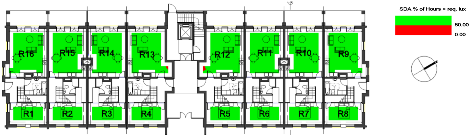
Figure 34: Block E Ground Floor sDA Pass/Fail Contours
