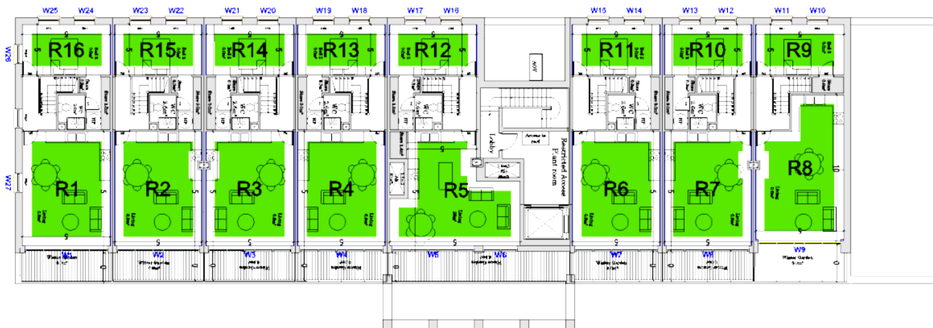
Figure 41: Block A/B Fourth Floor sDA Pass/Fail Contour
