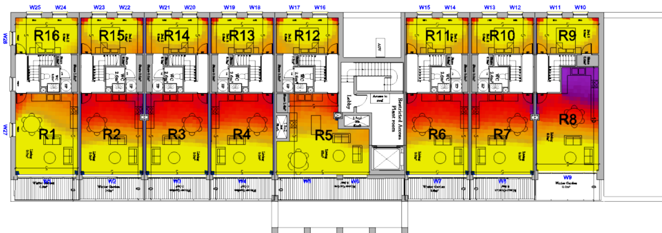
Figure 26: Block A/B Fourth Floor DF Contours
