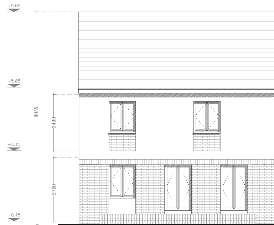
House Type D - Detached Side (Street) Elevation
