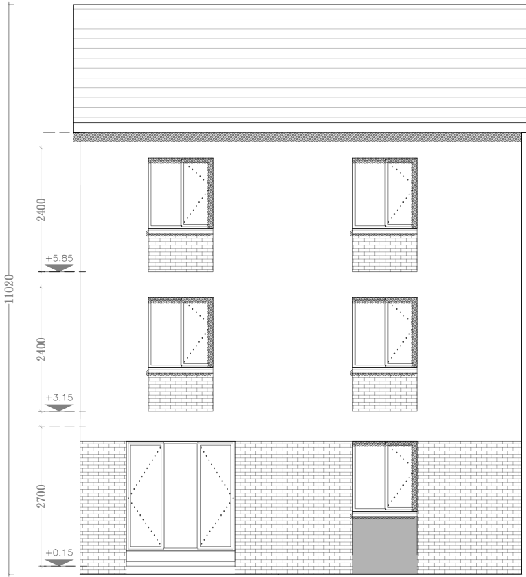
House Type N1 Side/ Street Elevation
