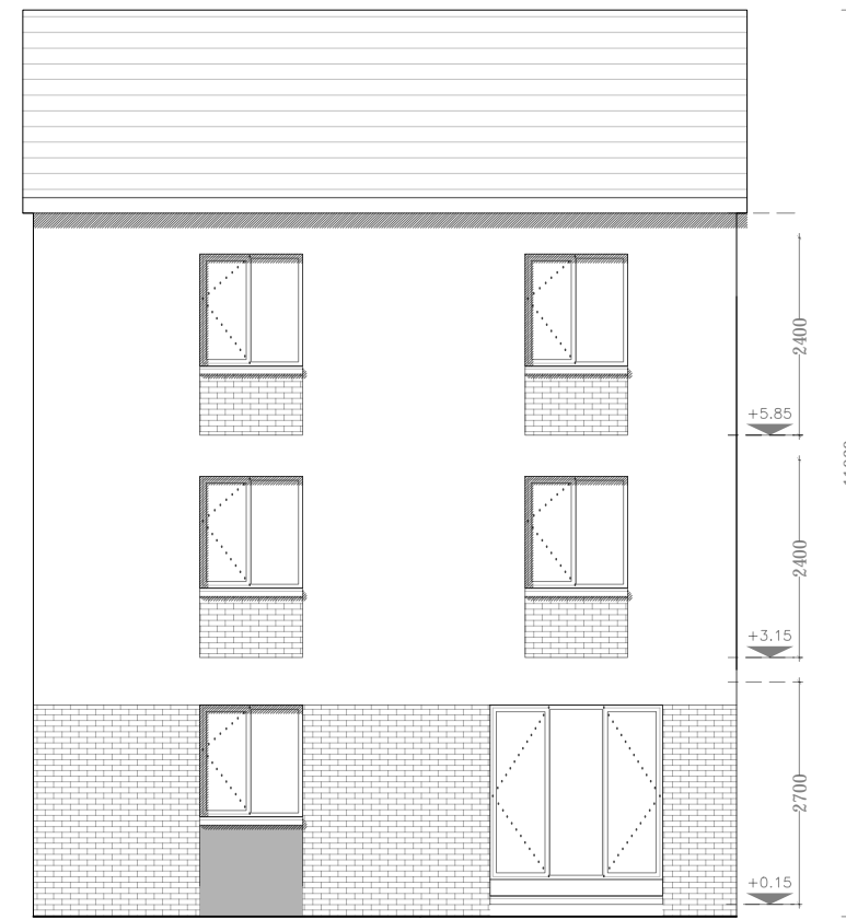
House Type N Side/ Street Elevation
