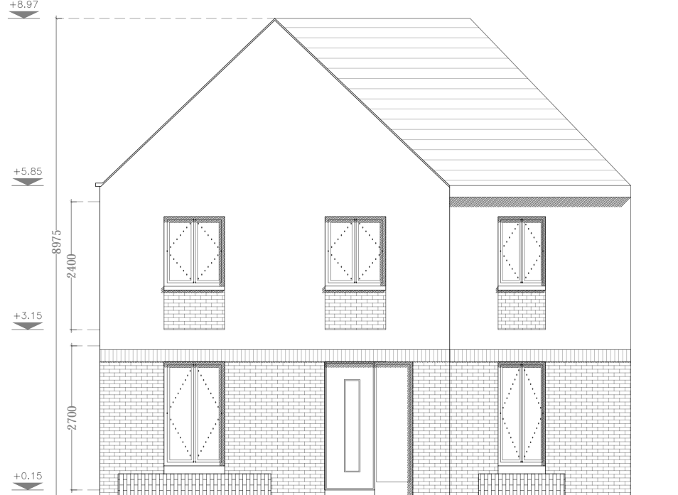
House Type P Front (Entrance) Elevation
