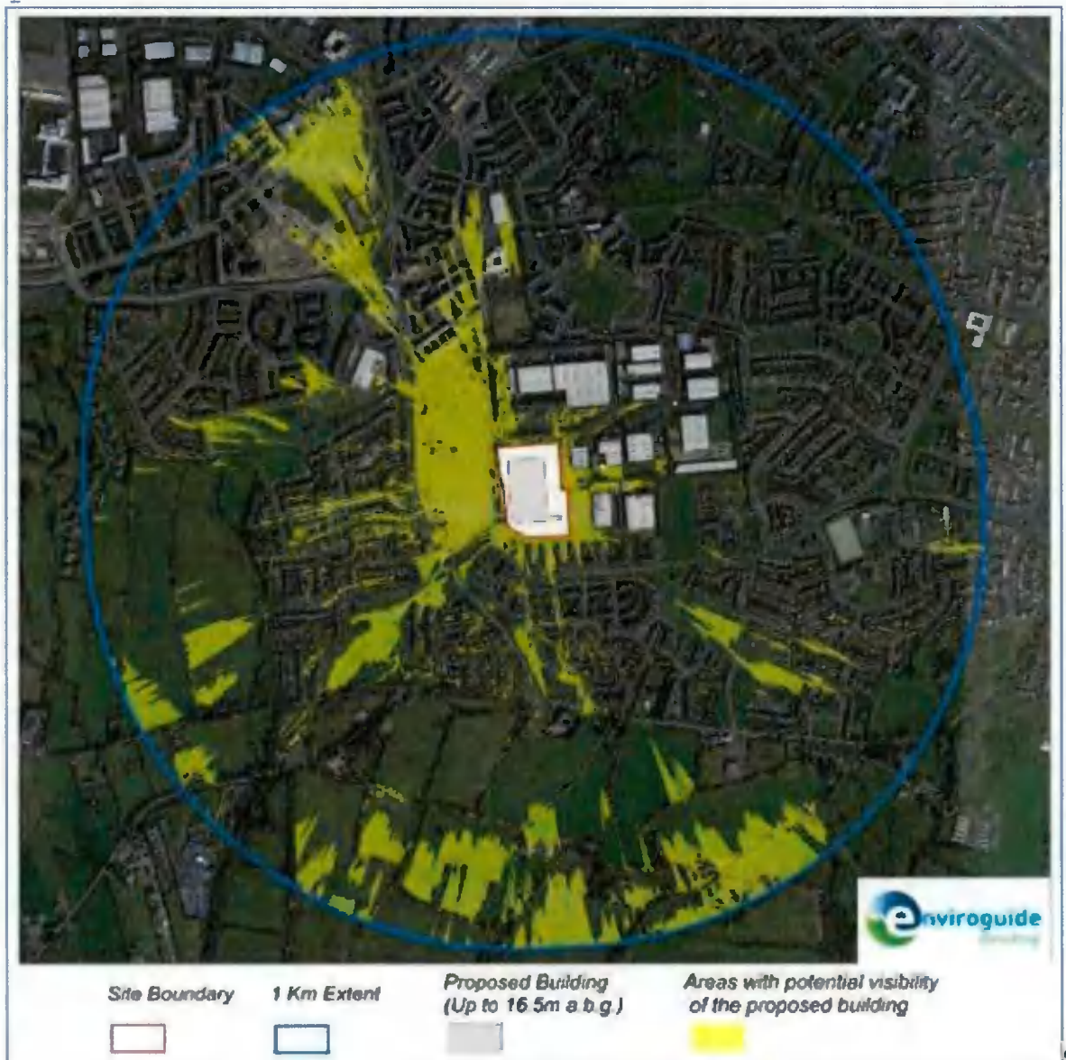
Figure 3 - Modified DSM-based Zone of Theoretical Visibility Map showing ground level visibility
