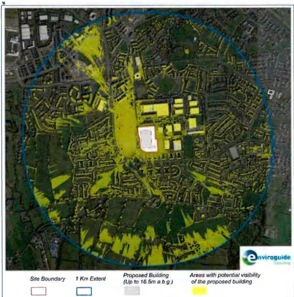
Figure 2 - Unmodified DSM-based Zone of Theoretical Visibility Map
