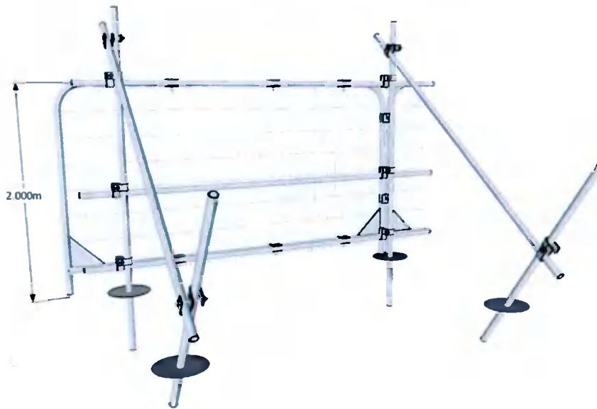
Figure 1. Protective fence specification
